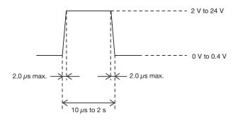
When trigger input polarity is negative
