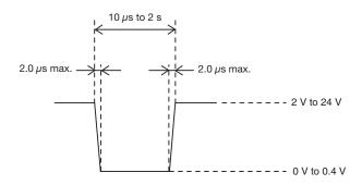
The voltage values described in the above diagram are the values when the terminating impedance is 10 k $\Omega$  or more.
