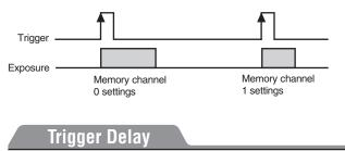
This function applies a trigger delay within the camera. Use it to synchronize trigger timing when the trigger signal is offset from the desired object exposure timing.
