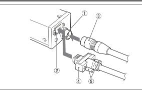
Connect the camera cable to the DC IN connector and the LAN cable to the RJ45 connector respectively. When you connect the LAN cable, turn the two fastening screws on the connector to secure the cable tightly.
