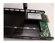
5 Holding the new M.2 module label-side up and at an angle, insert the module contact pins into the module slot.
