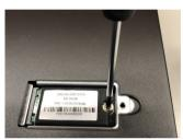
4 Holding the new M.2 module label-side up and at an angle, insert the module contact pins into the module slot and press the module down, aligning the notch with the inner screw location.
