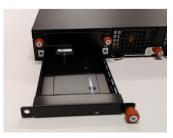
Use a PH1 screwdriver to remove the inner screw that holds the Λ existing M.2 module in place and then remove the module.
