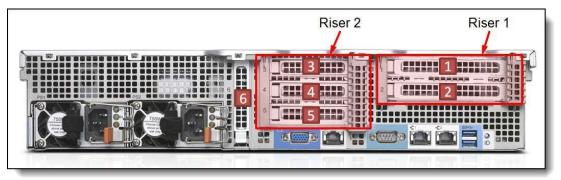
Figure 7. Slot numbering
