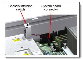
Figure 8. Chassis intrusion switch
