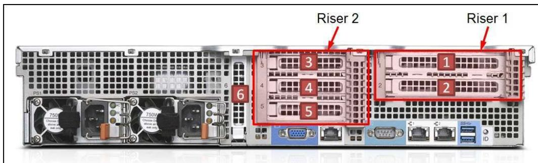
Figure 7. Slot numbering
