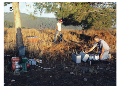
Early radar units were bulky and cumbersome. In relatively open areas, mobile surveys were conducted towing the antenna behind a vehicle (A). In more inaccessible areas, the GPR unit had to be carried in and powered off a generator with the antenna limited to a 30 m search radius (B).
