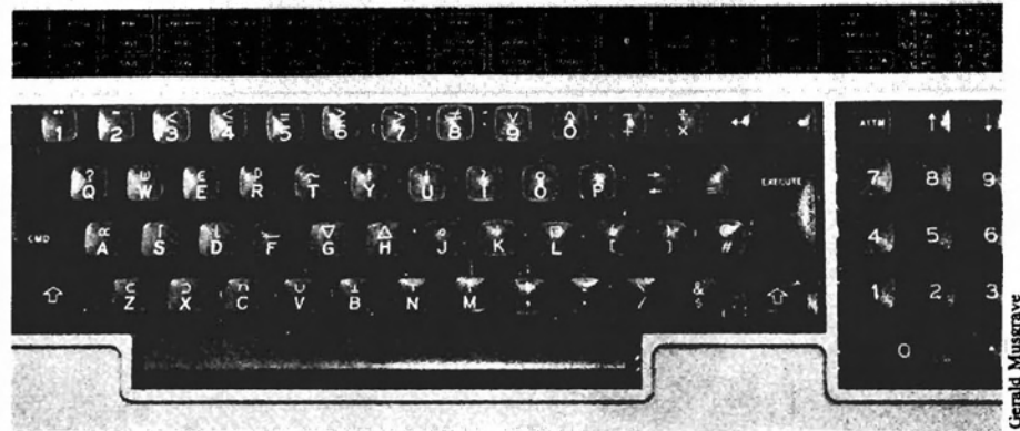
Figure 2.1 IBM 5120 desktop computer showing the APL character set, numeric pad, and special function keys.
