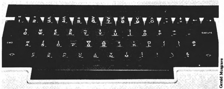
IBM 5120 showing keyboard characters that can be entered using the command key.
