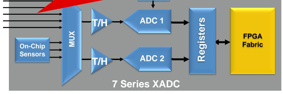
Note: Auxiliary channels 6, 7, 13, 14, and 15 are not supported on Kintex-7 devices
