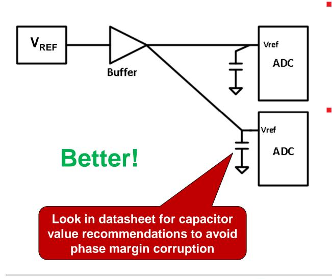
One reference capacitor is required at each ADC
