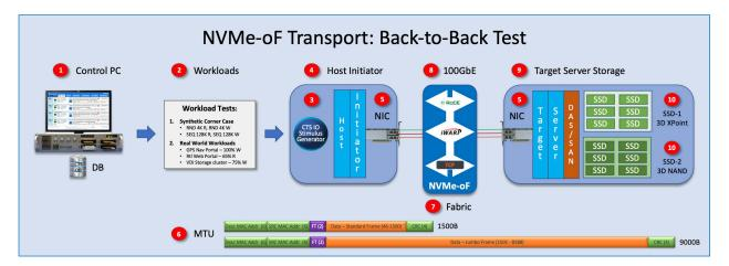
Figure 6 – Back-to-Back Test Topology
