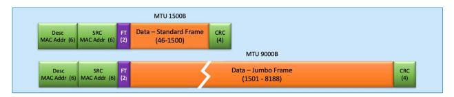
Figure 4 – MTU Frame Size: Standard 1500B v Jumbo 9000B
