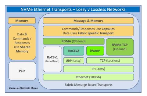
Figure 2 – NVMe Ethernet Transports: UDP v TCP
