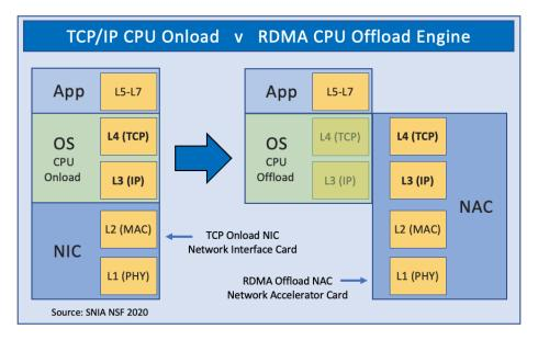
Figure 3 – Onload v Offload Engines
