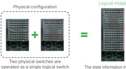
The state information including the configuration management routing table are shared using a single Cisco IOS and a single configuration file.
