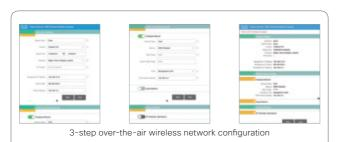
In the Cisco Mobility Express Solution, one access point (AP), running the Cisco Mobility Express wireless controller, is designated as the master AP. Other access points, referred to as subordinate APs, associate to this master AP. The master AP operates as a wireless controller, to manage and control the subordinate APs, and also operates as an access point to serve clients. The subordinate APs behave as normal lightweight access points to serve clients.
