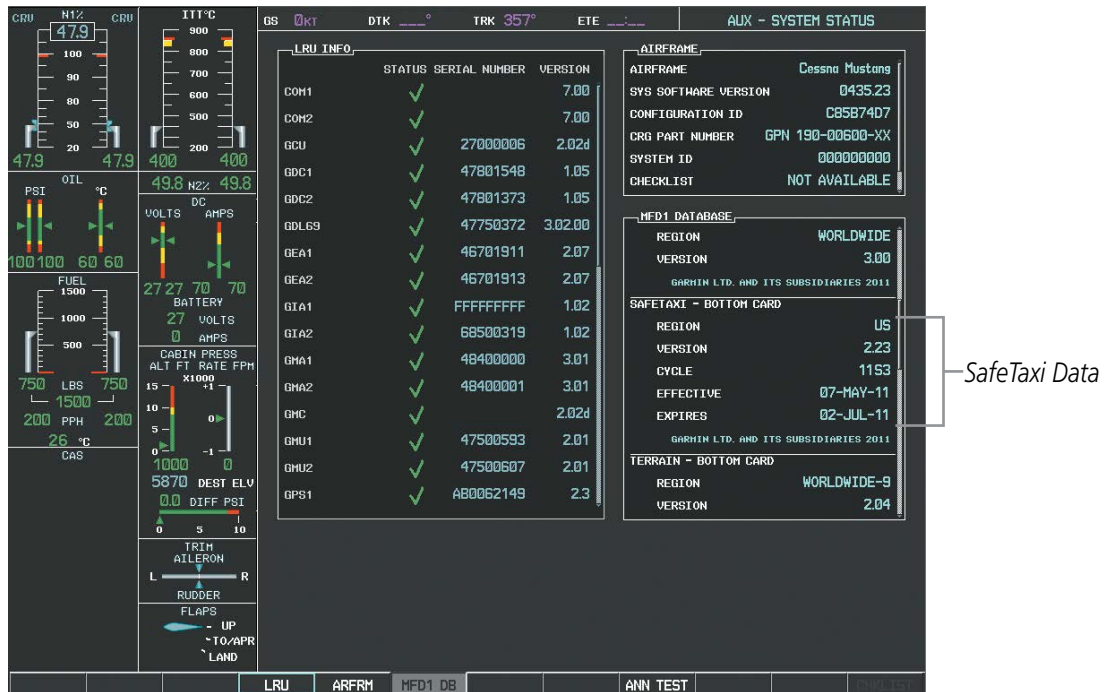
Figure 8-18 AUX – System Status Page, SafeTaxi Current Information
