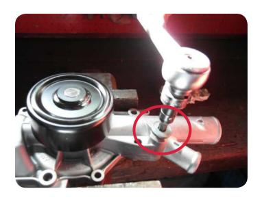
1) Tighten the accessory idler bolt into the bore. It is not necessary to use a new bolt to carry out this step.
