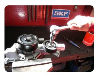
3) Install the new VKM 31041 idler and tighten to the vehicle manufacturers recommended torque setting.
