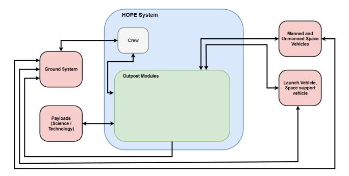
Figure 3.2 HOPE functional diagram
