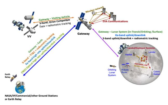
Figure 1.3 Gateway communications architecture [7]
