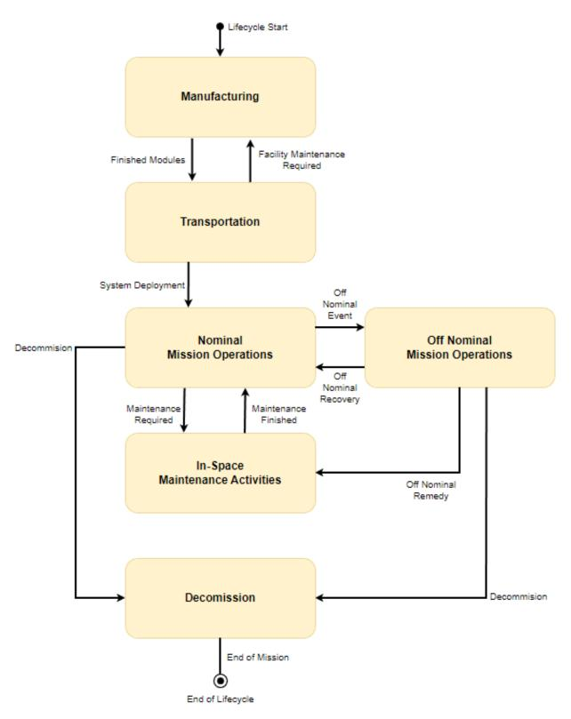
Figure 3.4 HOPE program level state machine diagram
