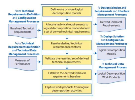
Figure 3.1 logical decomposition process [29]
