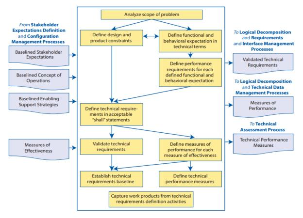
Figure 2.7 requirements definition process [29]
