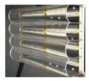
Figure 1.4 demonstration unit, stretched lens array for deep space applications [14]
