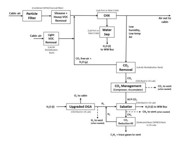
Figure 2.3 ISS Air String operational concept [31]
