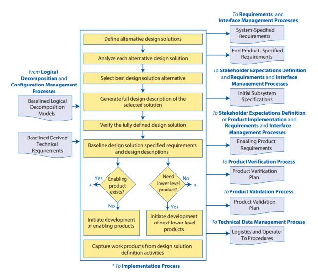
Figure 4.1 design solution definition process [29]
