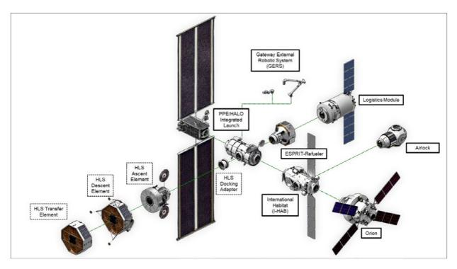
Figure 2.1 expanded view of the Lunar Gateway with optional configurations [30]
