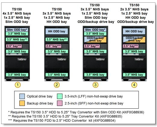
Figure 5. Internal storage configurations
