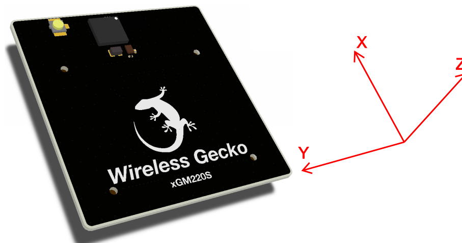
Figure 6.2. Illustration of Reference Planes with a Radio Board Plugged into the Wireless Starter Kit Mainboard
