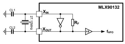
Figure 15: Typical application with a 27.12MHz crystal
