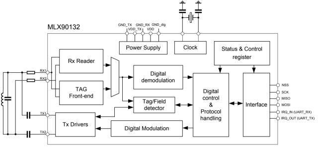
Figure 2: MLX90132 simplified block diagram
