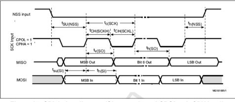
Figure 14: SPI timing diagram (Slave mode and CPOL = 1, CPHA = 1)
