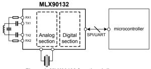
Figure 1: MLX90132 functional diagram
