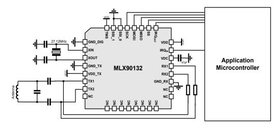
Figure 12: MLX90132 application schematic
