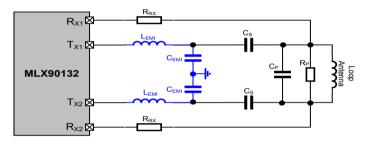
Figure 11: External antenna matching network
