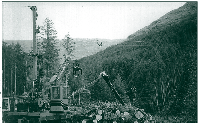
Whole-tree harvesting by cable crane
