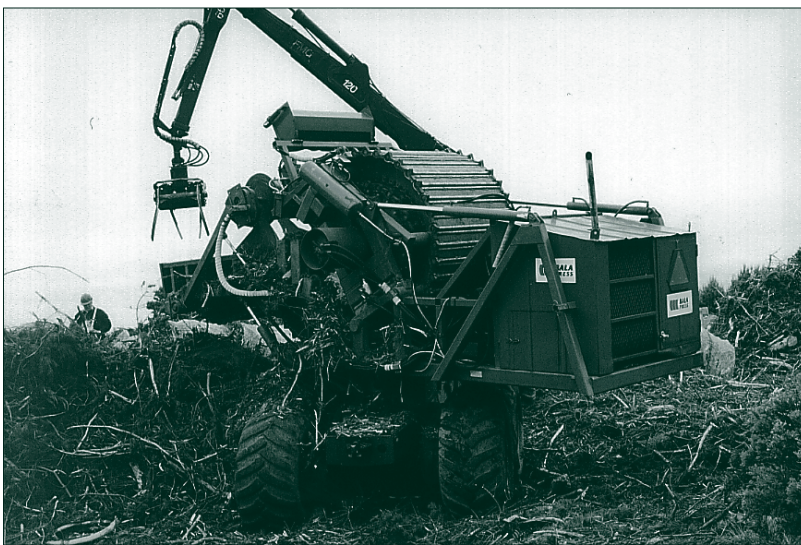
Second-pass residue harvesting – baling at the forest landing
