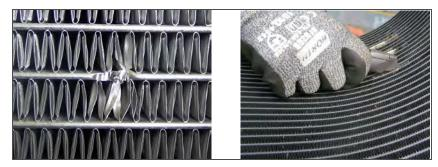
4. Using needle nose pliers, carefully remove the fins from the damaged area above and below the tube needing repair. The fins to be removed should be approximately 1/2" of fin material from each side of the repair location.
