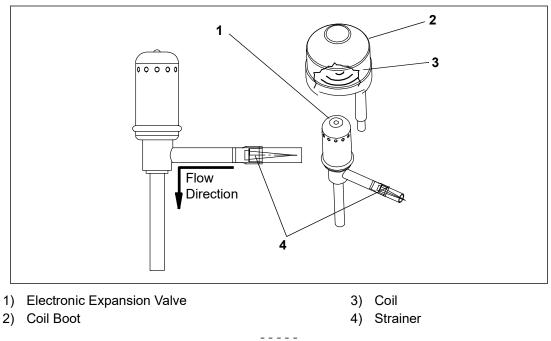
Figure 7.13 Electronic Expansion Valve (EEV)
