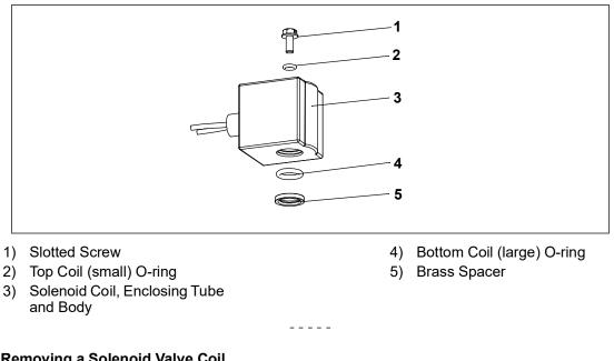
Figure 7.14 Coil View of Economizer Solenoid Valve (ESV)
