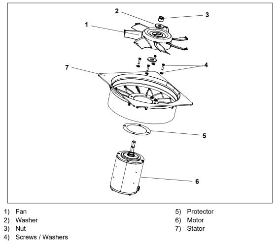
Figure 7.11 Evaporator Fan Assembly
