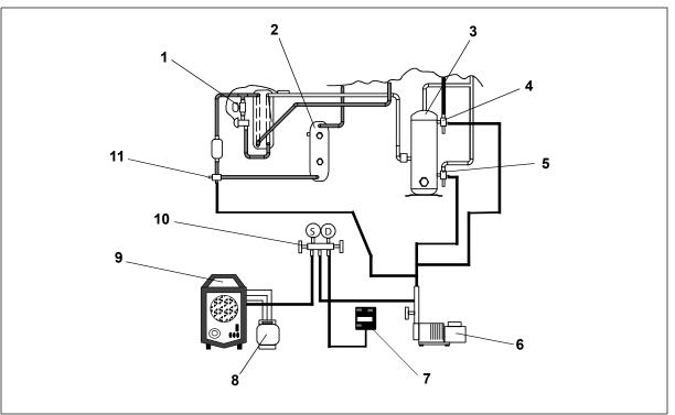
Figure 7.4 Refrigeration System Service Connections
