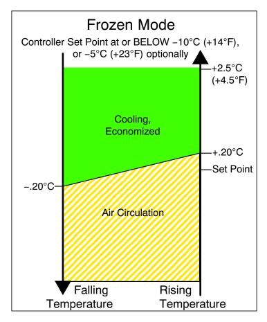
Figure 4.6 Controller Operation - Frozen Mode
