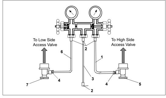
Figure 7.2 Manifold Gauge / Hose Set
