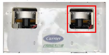
Figure 7.22 Removing Evaporator Motor
