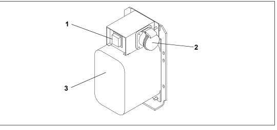
Figure 5.1 Autotransformer
