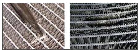
5. Remove dirt from the surface around the leak point with a soft bristle brush and water. Then wash off any residual oil with alcohol. Allow the surfaces to fully air dry.
