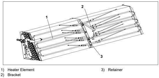
Figure 7.10 Heater Arrangement
