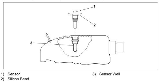
Figure 7.36 Compressor Discharge Temperature Sensor
