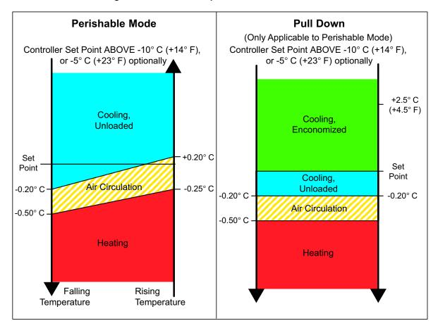
Figure 4.3 Controller Operation - Perishable Mode
