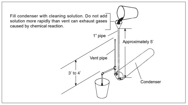
Figure 7.9 Water-Cooled Condenser Cleaning - Gravity Circulation
