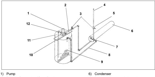
Figure 7.8 Water-Cooled Condenser Cleaning - Forced Circulation
