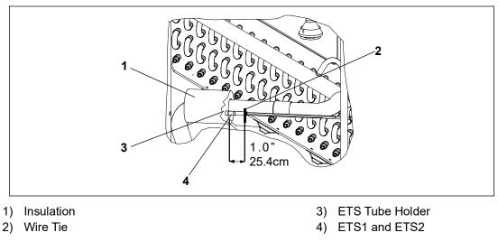
Figure 7.35 ETS1/ETS2 Positioning
