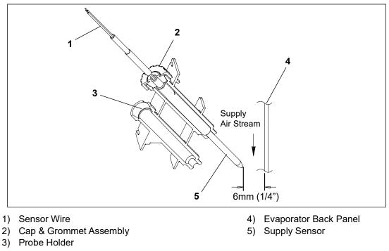
Figure 7.33 STS/SRS Positioning
