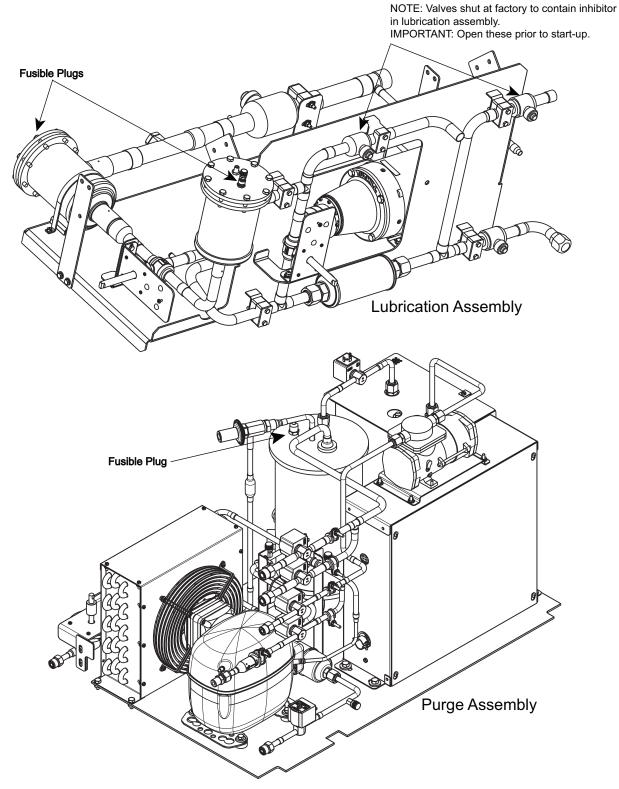
Fig. 10 — Location of Fusible Plugs in Lubrication Assembly and Purge Assembly
