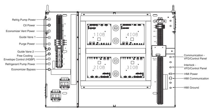
Fig. 21 — Control Panel, IOB Layer
