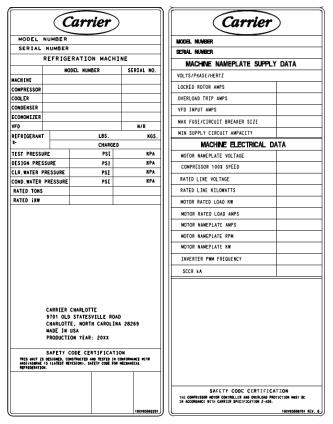
Fig. 1 — 19DV Refrigeration Machine Nameplate
