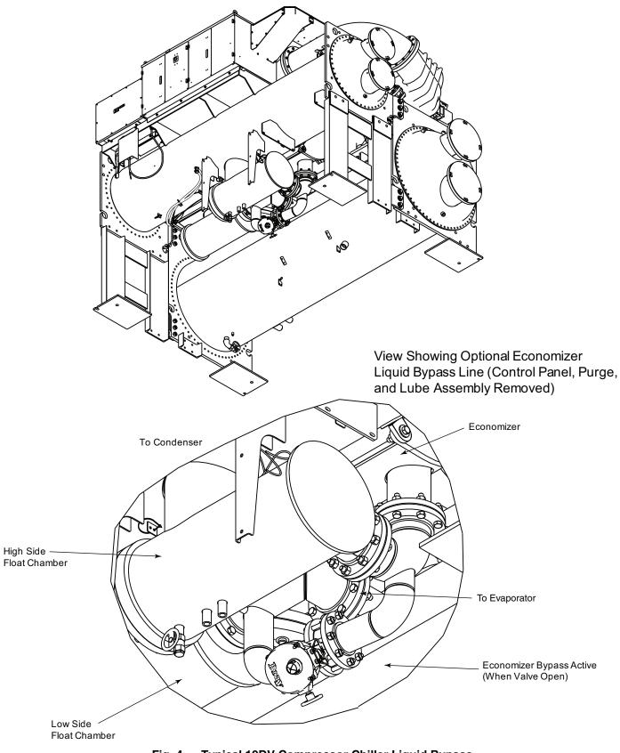
Fig. 4 — Typical 19DV Compressor Chiller Liquid Bypass
