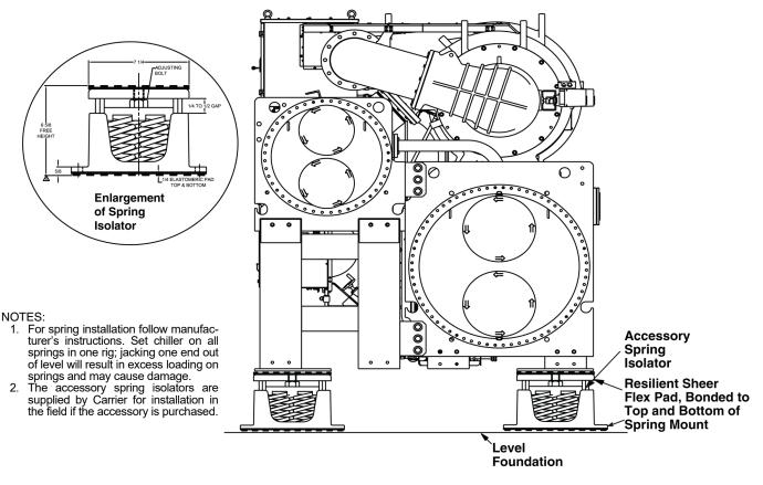
Fig. 12 — 19DV Accessory Spring Isolation (Shown with Accessory Soleplates)
