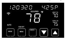
The center portion of the screen displays the current space temperature in whole degrees. The default temperature scale is °F, but can be changed to °C in the *Installer settings* (page 31).
