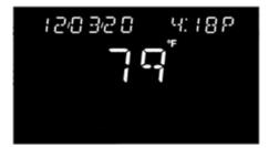
The banner scrolls through date and time, humidity, outdoor air temperature, if configured, and any active faults or system events. The room temperature is prominently displayed.
