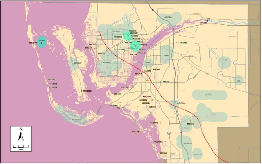
**Figure F-48.** Estimated position of the saltwater interface within the Mid-Hawthorn aquifer in Lee County in April–May 2009. The figure number labels refer to Figure F-49 through Figure F-58, which show chloride levels for the indicated wells.
