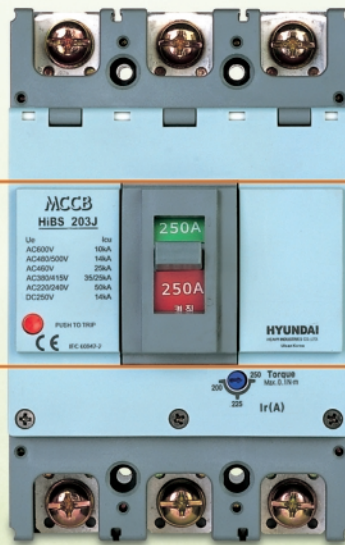
250AF Adjustable thermal In from 100 to 250A Icu = 18 / 25 / 35kA at 415V 2, 3, 4 pole Adjustable-thermal and fixed-magnetic trip unit
