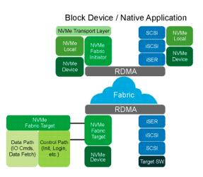
The embedded PCIe switch enables customers to build standalone storage or Machine Learning appliances. As with the earlier generations of ConnectX adapters, standard block and file access protocols leverage RoCE for high-performance storage access. A consolidated compute and storage network achieves significant cost-performance advantages over multi-fabric networks.
