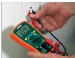
Displays AC Voltage of an outlet receptacle
