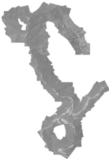
Fig. 6.11. 2D Surface Map build by Robot with 50 particles.
