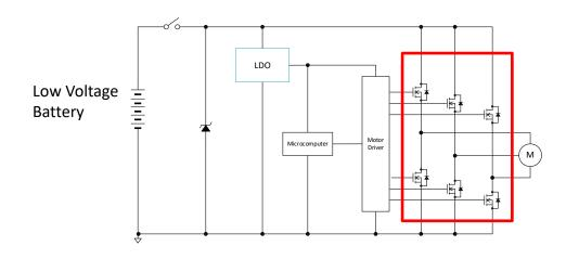
$V_{DSS}$  = 40 V to 300 V,  $I_{D}$  = ±20 A to ±100 A
