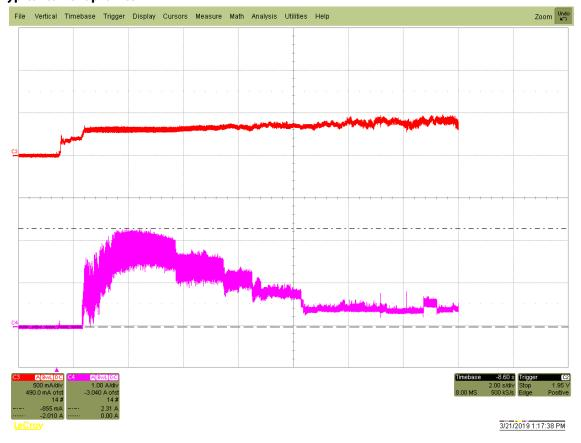
Figure 4. 2TB Typical startup and operation current profile
