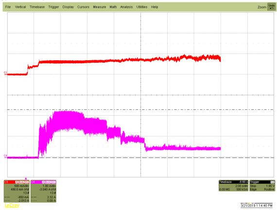
Figure 3. 4TB Typical startup and operation current profile
