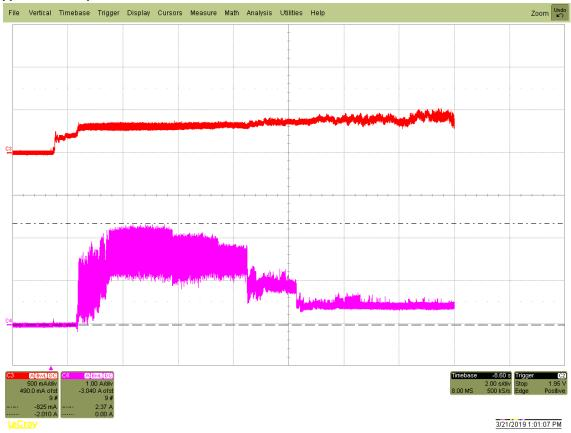
Figure 2. 6TB Typical startup and operation current profile
