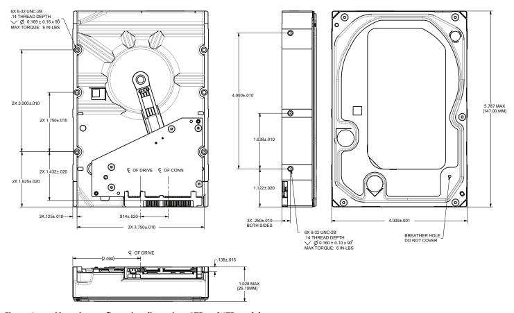
Figure 6. Mounting configuration dimensions 8TB and 6TB models
