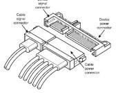
Figure 5. Attaching SATA cabling
