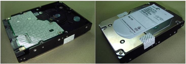
Figure 8. Example of FIPS tamper evidence labels.
