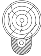
METHOD 2 WOOD MOULDING OF 1 1/2" MINIMUM THICKNESS
