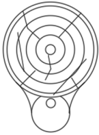
METHOD 1 IMPREGNATED FIBER CONDUIT OF 1/4" MINIMUM THICKNESS
