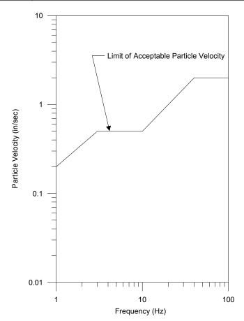
Figure 1 - Vibration Criteria (adapted from AASHTO R8-96)
