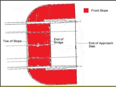
Figure - Front Slope Definition
