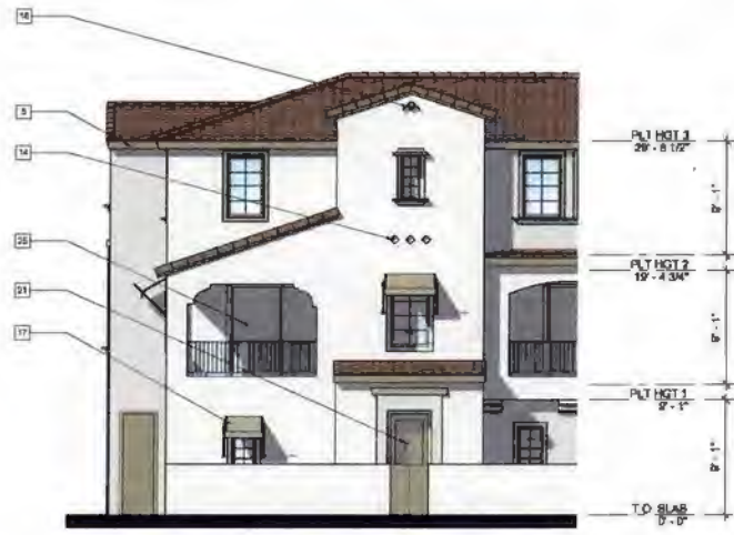
2 Partial Front Elevation - A - Visitable Unit 3/16" = 1'-0"
