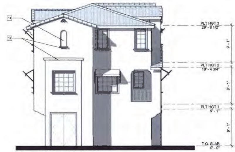
3 Left Elevation - A Four Plex 3/16" = 1'-0"
