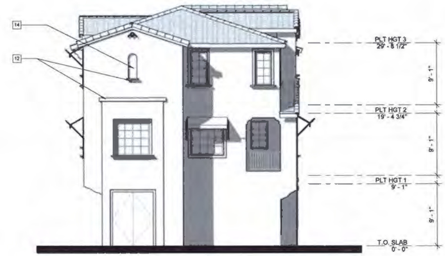
3 Left Side Elevation - A 3/16" = 1'-0"
