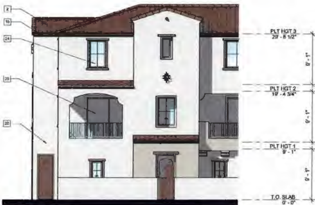
2 Partial Front Elevation - B - Visitable Unit 3/16" = 1'-0"
