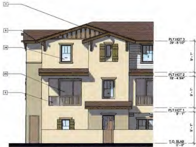
2 Partial Front Elevation - C - Visitable Unit 3/16" = 1'-0"
