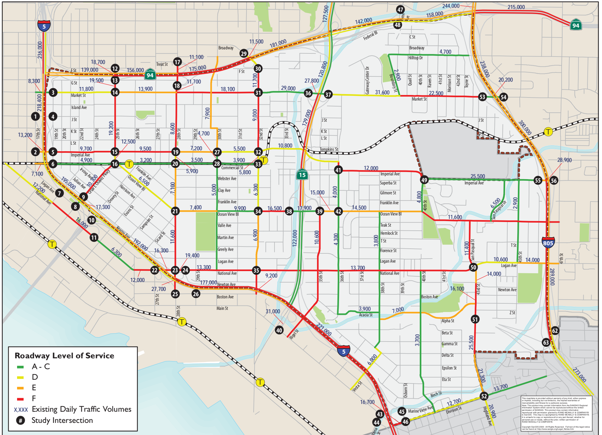
Figure 5.2-13: Southeastern San Diego Preferred Plan Roadway Traffic Volumes and Level of Service
