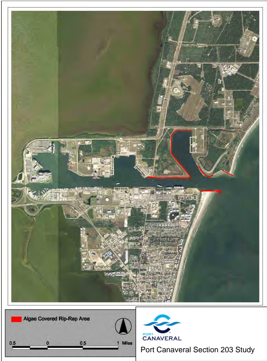
Figure 2-10 Algae Covered Rip-Rap
