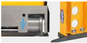
Setting out and clamping = working position
