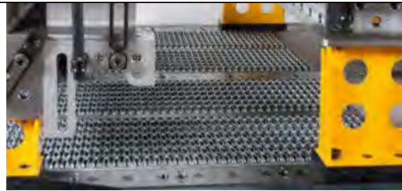
The set-up heights can be adapted to the workpiece by simply exchanging the legs.
