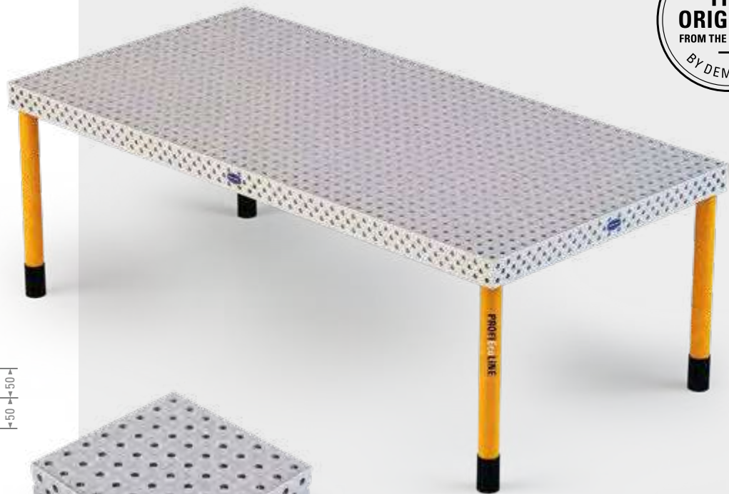
Three-row bore pattern on the table side plates with D16 system bores in a 50 mm grid in the top, middle and bottom rows
