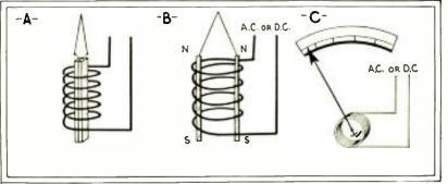
The principle of operation of the iron-vane movement used in A.C. meters is shown above.
