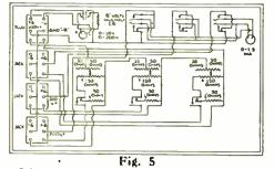
Schematic circuit of the condenser microphone mixer illustrated in Fig. A.
