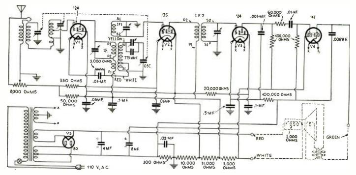
Schematic circuit of the Models 99 60-cycle, and 99X 25-cycle superheterodyne receivers. yne receivers. A band-selector precedes the first-detector-oscillator, V1, known, as the dial is calibrated to read directly in broadcast band The signal frequency settings of the service oscillator must be accurately frequencies.
