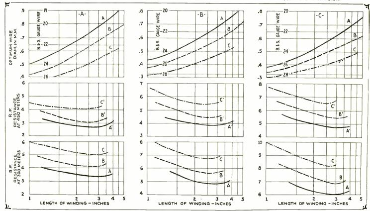
Figure 4, upper row. The curves A, B, and C indicate the optimum size wire for various winding lengths, inductance and coil diameters. Curves A, B, and C are coils 3 ins., 2½ ins., and 2 ins. in diameter, respectively. The three rows A, B, and C are for coils of different lengths; A to be used with .0005-mf, tuning condensers, B with .00035-mf, and C with .00025-mf, condensers.
