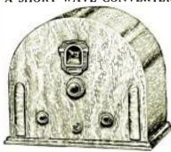
The short wave converter that has its own fower supply, making operation independent of the type of receiver used.
