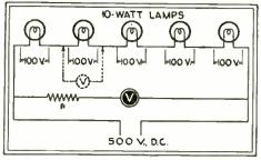
The voltage drop across each lamp should be 100 volts, if five 10-west lamps are connected across a 500 volt source,
