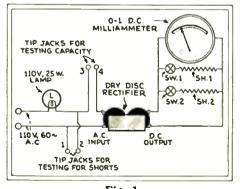
Circuit connections of the capacity meter. A dry-disc rectifier in conjunction with a D.C. meter is used for measuring values between .005- and 10 mf.
