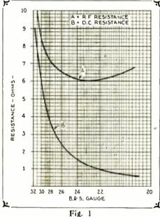
Note that for the smaller gauge wire the A.C. resistance of a coil may be several times its D.C. resistance.
