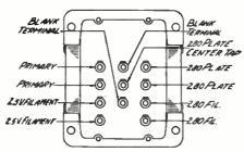
Power transformer terminal connections of the Model 99 Chassis.
