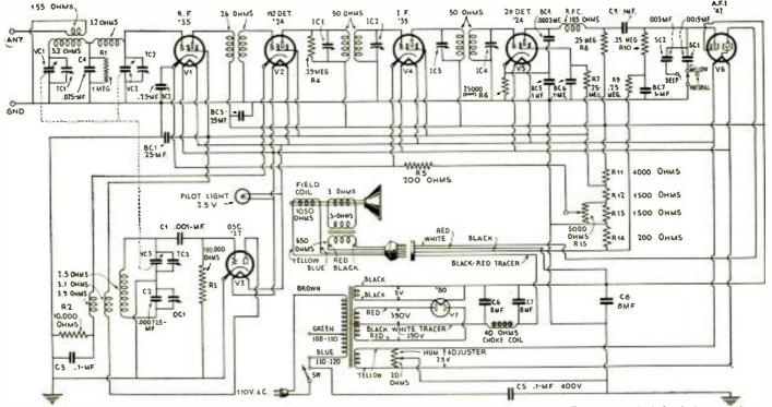
Schematic circuit of the new Kolster-International Models K-60 60-cycle, and K-62 25-cycle radio receivers. The antenna is inductively-coupled to a bund-selector preceding a single-stage signal-frequency amplifier using a type '35 variable-mu tube. The tuning characteristic is flat-top. The set must not be turned on when the reproducer is not plugged into circuit. Power detectors are used.
