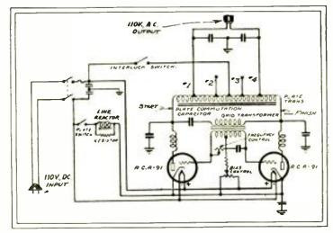
The schematic diagram of the Thyratron Inverter is shown above. When 110 volts D.C. are applied to the input, 110 volts A.C. is obtained at the output,
