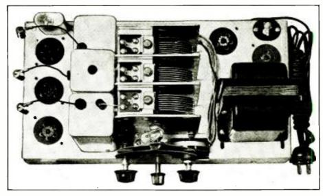
Parts arrangement on top of the Model 99 receiver chassis. To prevent circuit oscillation it is essential to keep all leads short and in correct location. For good operation, an important item is good tubes.
