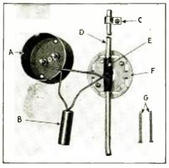
Fig. J At A is shown the surface box, at B the "taplet," as C the Cabloy clamps, at D the Cabloy, at E the tap to the outlet box, at F the base of the surface box, and at G the mounting screws.
