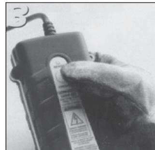
3 Press and hold control unit switch and wait for the ignition
