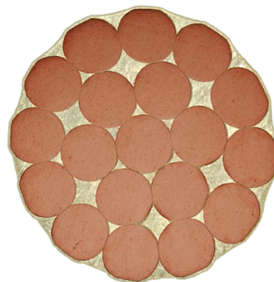
Figure 08-8 Solder Penetration on Tinned Wire
