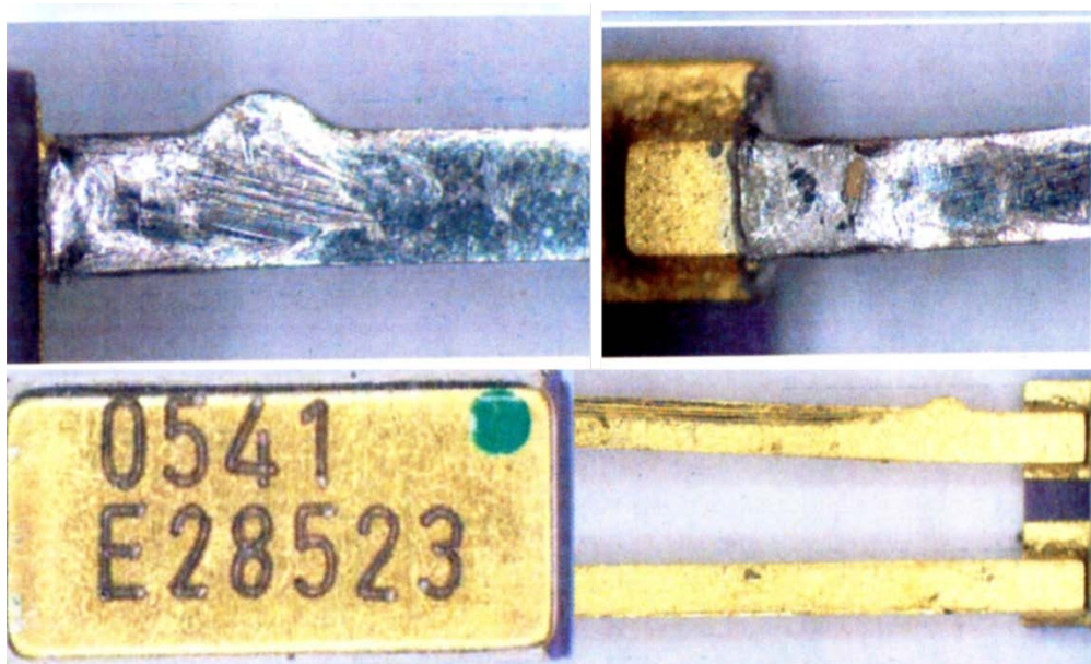
Figure 03-28: Component leads showing either evidence of previous component use and retinning (top) or incorrect lead finish (bottom).
