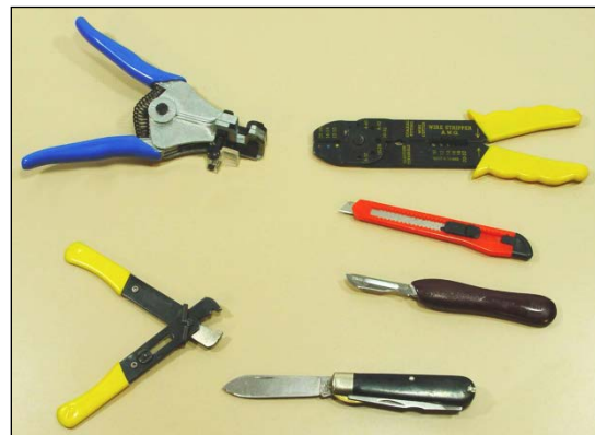
Figure 08-7 Strippers NOT Approved for 2M Repair
