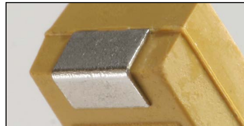
Figure 18-2 Inward L-Shaped Ribbon Leads
