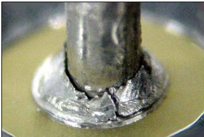
Figure 05-8 Fractured Solder Joint
