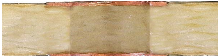
Figure 07-2 Double-Sided Non-Plated-Through Hole CCA (cross-section)
