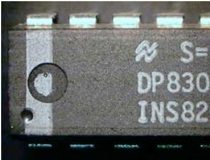
Figure 03-33: Suspect counterfeit component identified by a marking inside the indent.
