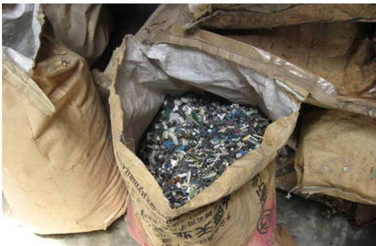
Figure 03-25: A bag full of harvested electronic components to be used in counterfeiting operations. Figure provided by SMT Corp.
