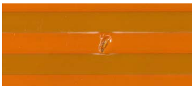
Figure 13-2 Flex Print Damage
