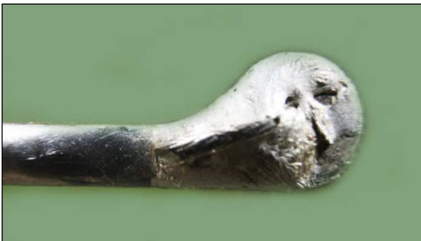
Figure 05-10 Heavily Oxidized Solder Joint
