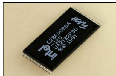
Figure 18-18 Type I Thin Small Outline Package
