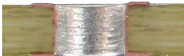
Figure 07-3 Double-Sided Plated-Through Hole CCA (cross-section)
