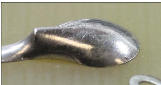
Figure 05-2 Convex Solder Fillet
