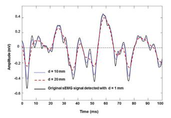
Fig. 12. Low-pass filtering effect for two different diameters of a circular electrode on a monopolar sEMG signal in time. The signal has been acquired with two pin electrodes having  $d=1\,\mathrm{mm}$  and has been filtered with the transfer functions depicted in Fig. 11. Observe the strong attenuation of the sharp peaks due to electrode size.
