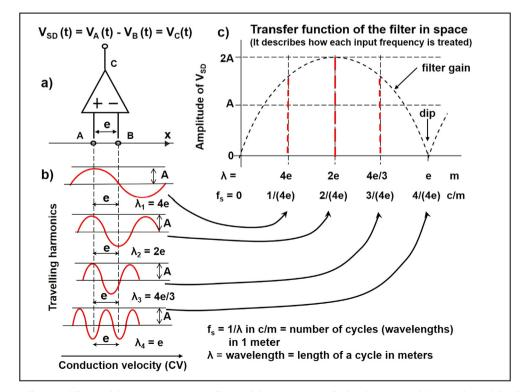
**Fig. 13.** Spatial filtering effect of a differential detection system. (a) Differential detection system, (b) four harmonics of the spatial signal distribution moving along x with velocity u. (c) Amplitudes of the four harmonics observed in point C (V<sub>SD</sub>).
