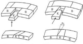
a) K segment inserted in radial direction
