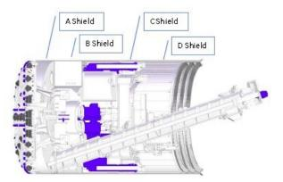
Figure 5. EPB shield configuration
