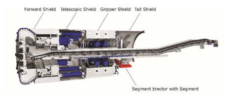
Figure 6. Shield configuration for double shield TBMs
