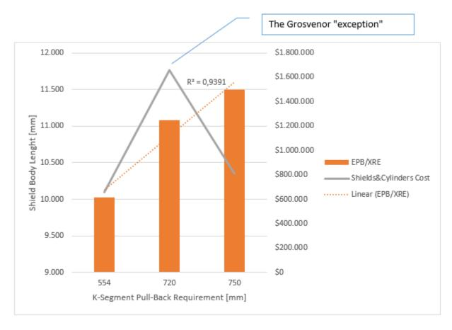
Figure 10. EPB segment width compared to shield body length and cost
