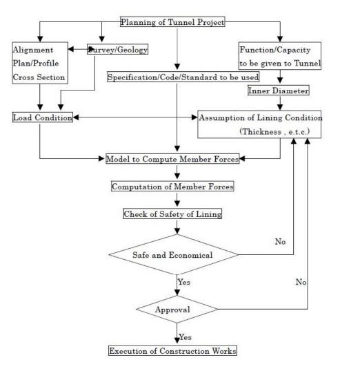
Figure1. Segment design workflow
