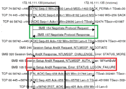
Fig.2. Message Sequence Chart of SMB Authentication Failure
