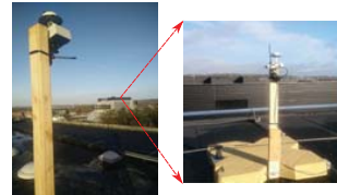
Fig. 6. ublox M8P base (left) and rover (right) mounted on rooftop of Aalborg University buildings. The spatial separation between the rooftop of base and rover is 160 m.
