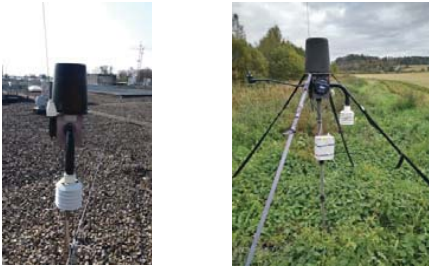
Fig. 4. Automatic Weather Station with RF1 module inside
