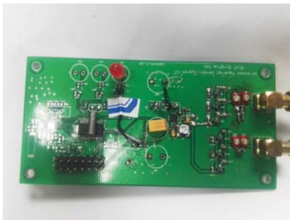
Fig. 8: The real prototype of triple double the voltage and twice double the current
