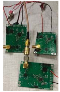
Fig. 2. Current consumption @3.1V for RF169MHz module with PA activated (leftmost) Hardware RF modules based on the wireless CC1125 device (rightmost).
