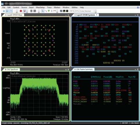
Fig. 2 Typical modulation channel VSA screen shot
