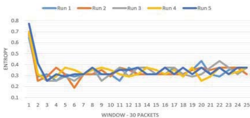
Fig. 10. Entropy fluctuations in network under botnet attack on one host – topology 2
