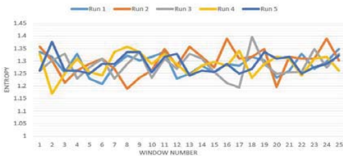
Fig. 5. Entropy in normal circumstances for experiment 2.
