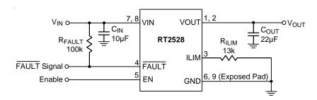
Note :  $R_{ILIM} = 13k\Omega$  for 2A Power Switch Operation
