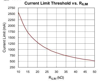
Figure 1. Current Limit Threshold vs. RILIM
