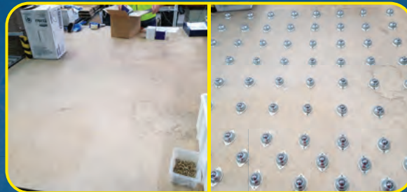
Stock transfer table refurbished with new rollers
