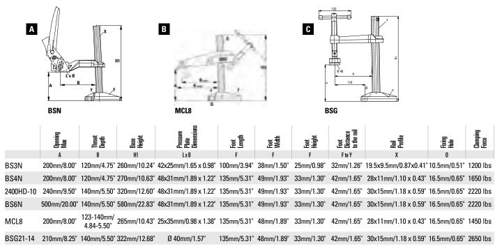
Note: Clamping force calculated at a height of 2-3" on a solid all-steel welding table platform
