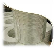
**EICOROV** - **510 MC** series is a multi-compatible single-end roving consisting of continuous **E-CR** glass fibers manufactured by the direct draw process and winding them on cylindrical package. The roving is treated with a special sizing system based on silanes which provides excellent performance with a wide variety of thermoset resins such as polyester, vinyl ester, epoxy etc.
