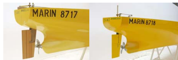
Figure 15 KVLCC models built by INSEAN, scale 1:45.71, left: KVLCC1, right: KVLCC2
