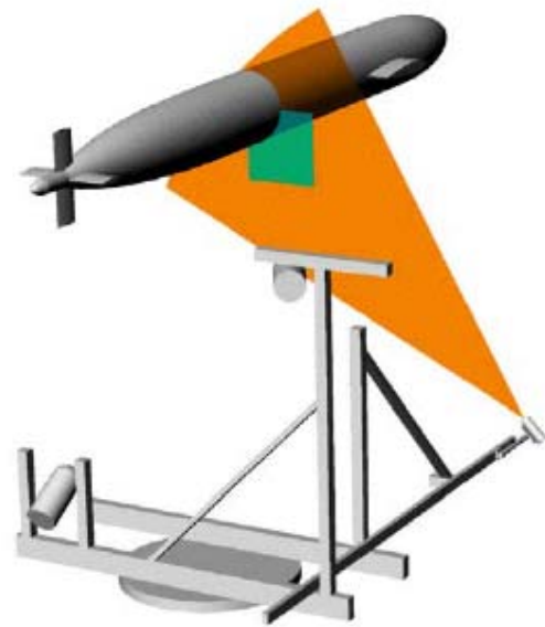
Figure 30 Earth fixed stereo PIV system for submarine static drift tests. (Atsavapranee et al 2004)
