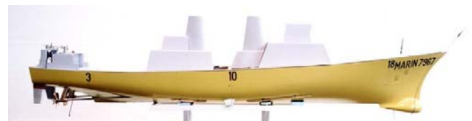
Figure 19 5415 model, built by MARIN, scale 1:30.48, appended hull
