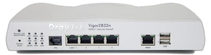
A 4-port Gigabit Ethernet switch on the LAN side provides high speed connectivity for your server, other local PCs or for uplink to a larger Ethernet switch. Comprehensive security features include content filtering, web application controls and an object based firewall management system.
