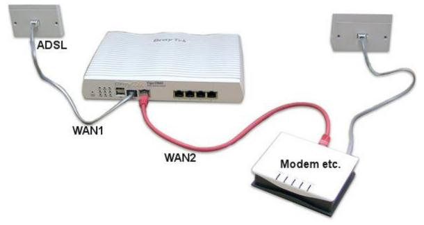
The Vigor 2832 can connect directly to an ADSL/ ADSL2+ line. WAN2 is a Gigabit Ethernet port and can connect to a secondary modem/connection, such as another ADSL or VDSL modem.
