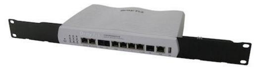
The RM1 Rackmount Bracket enables you to fit any Vigor2832 series router into a standard 19" rack or cabinet. The bracket takes up one rack slot (1U) and includes a cable retainer at the back to keep the power cord captive. The front mounted sockets of the router remain fully accessible. For wireless models, we then recommend extension aerials (or aerial extensions).
