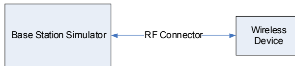
Figure 9-3 Power Measurement Setup
