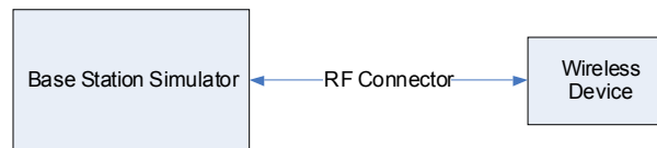
Figure 9-1 Power Measurement Setup
