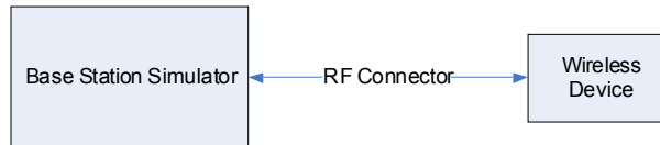
Figure 9-2 Power Measurement Setup
