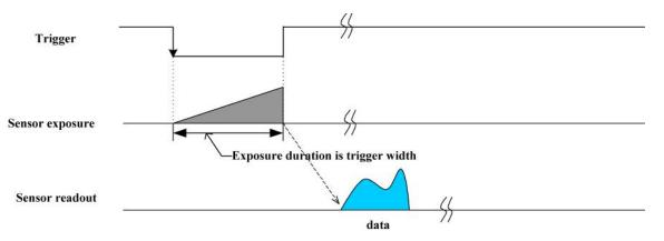
Figure 7.2: Trigger Mode 1 ("Bulb Shutter Mode")
