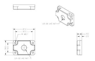
Figure 4.2: Tripod Adapter Dimensional Diagram
