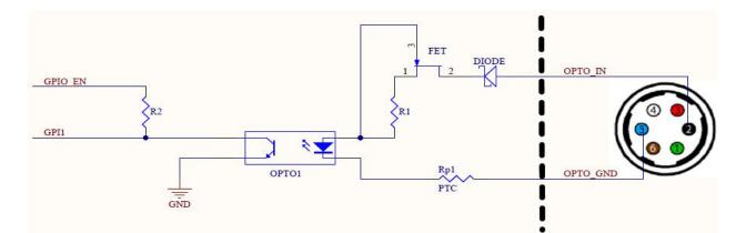
Figure 6.2: Opto-isolated input circuit
