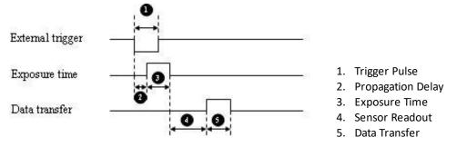
Figure 7.6: External trigger timing characteristics
