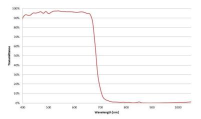
Figure 4.4: IR filter transmittance graph
