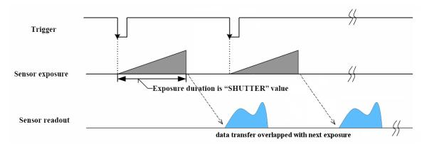
Figure 7.4: Trigger Mode 14 ("Overlapped Exposure/Readout Mode")
