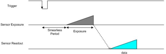
Figure 7.3: Trigger Mode 13 ("Low Smear Trigger Mode")
