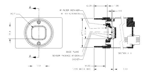
Figure 4.3: Example C-mount Cross Section
