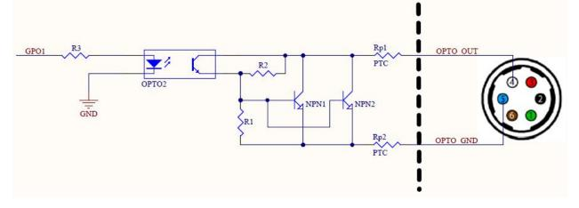
Figure 6.3: Opto-isolated output circuit
