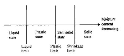
Figure 1.21 Consistency of cohesive soils.
