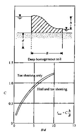
Figure 5.40 Critical exit gradient [Eq. (5.172)].
