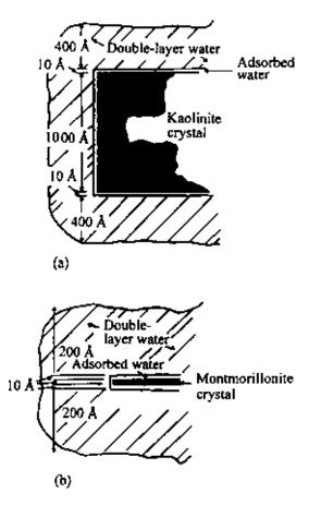
Figure 1.8 Clay water (a) typical kaolinite particle, 10,000 by 1000 Å and (b) typical montmorillonite particle, 1000 by 10 Å (after Lambe, 1960).
