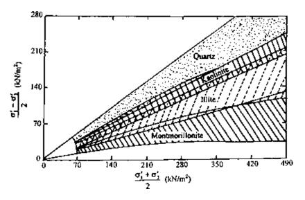
Figure 7.20 Modified Mohr's failure envelope for quartz and clay minerals (after Olson, 1974).
