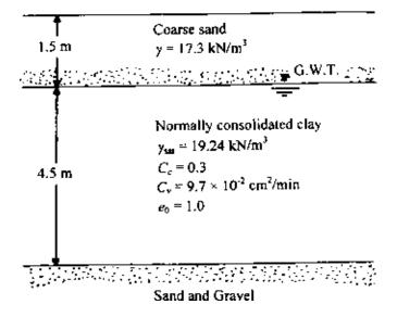
Figure 8.31 Soil profile for precompression.
