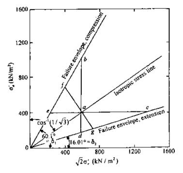
Figure 7.44 Stress paths for tests 1-6 in Example 7.4.
