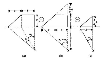
Figure 3.14 Vertical stress due to embankment loading.
