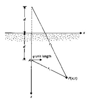
Figure 3.8 Horizontal line load inside a semi-infinite mass.
