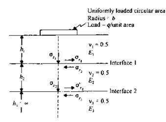
Figure 3.30 Uniformly loaded circular area on a three-layered medium.
