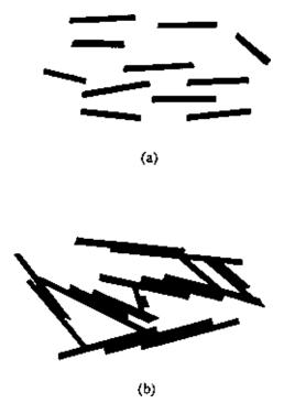
Figure 1.19 (a) Dispersion and (b) flocculation of clay.
