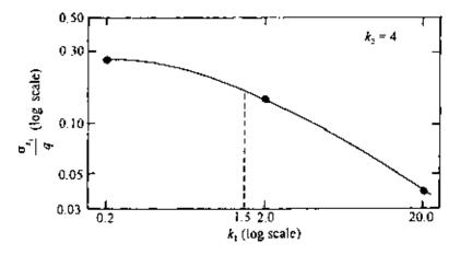
Figure 3.32 Plot of  $\sigma_{z_1}/q$  against  $k_1(k_2 = 4)$ .
