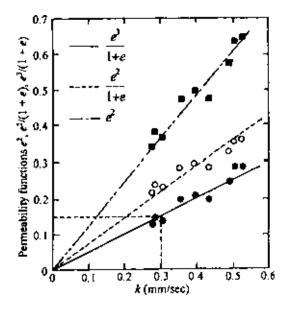
Figure 5.7 Plot of k against permeability function for Madison sand.
