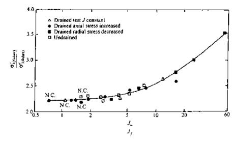
Figure 7.52 Plot of  $\sigma'_{1(failure)}/\sigma'_{3(failure)}$  against  $J_m/J_f$  for Weald clay—compression tests (after Henkel, 1960).
