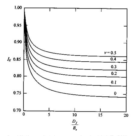
Figure 8.10 Variation of embedment correction factor  $I_{\rm E}$  with  $D_{\rm f}/B_{\rm e}$  [Eq. (8.30)].
