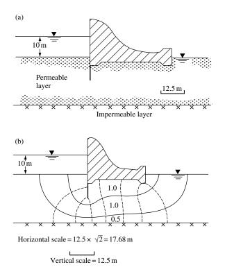
Figure 5.31 Construction of flow net under a dam.
