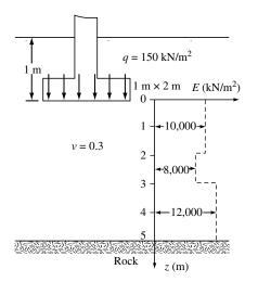
Figure 8.5 Elastic settlement for a rigid shallow foundation.
