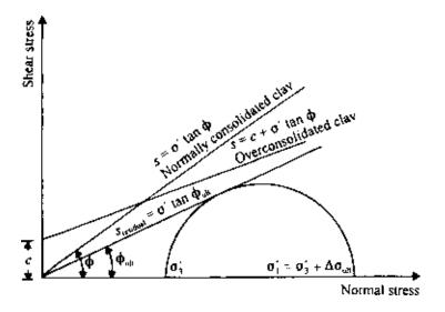
Figure 7.23 Residual shear strength of clay.
