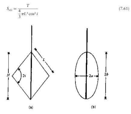
Figure 7.67 (a) Triangular vane and (b) Elliptical vane.
