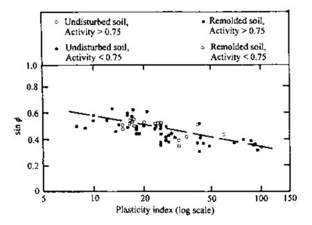
Figure 7.32 Relationship between sin  $\phi$  and plasticity index for normally consolidated clays (after Kenney, 1959).
