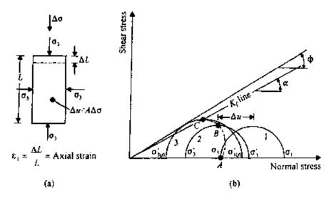
Figure 7.41 Stress path for consolidated undrained triaxial test.
