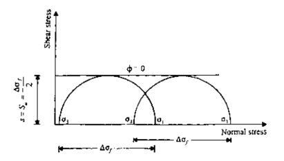
Figure 7.27 Unconsolidated undrained triaxial test.
