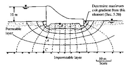
Figure 5.27 Flow net under a dam.
