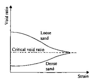
Figure 7.11 Definition of critical void ratio.
