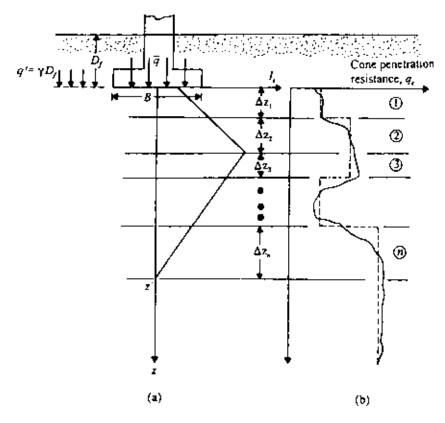
Figure 8.12 Calculation of S<sub>e</sub> from strain influence factor.
