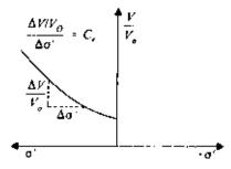
Figure 4.9 Definition of  $C_{e}$ : coefficient of volume expansion under uniaxial loading.
