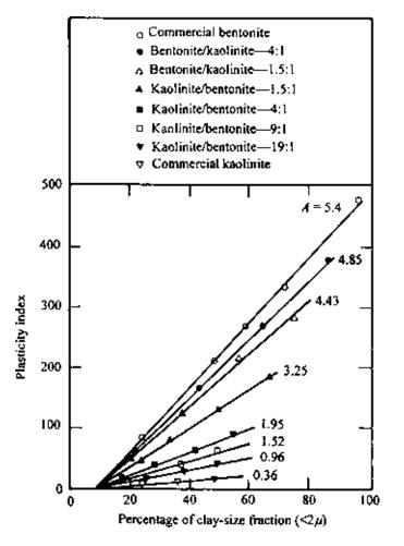
*Figure 1.27* Relationship between plasticity index and clay-size fraction by weight for kaolinite/bentonite clay mixtures (after Seed *et al.*, 1964a).
