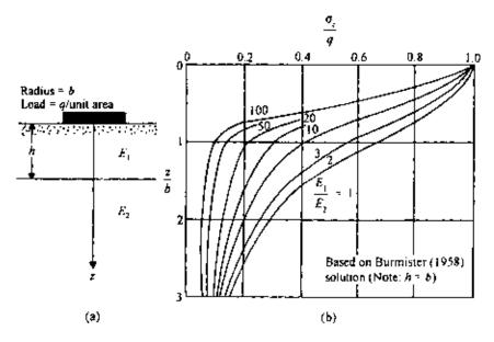
Figure 3.29 (a) Uniformly loaded circular area in a two-layered soil  $E_1 > E_2$  and (b) Vertical stress below the centerline of a uniformly loaded circular area.
