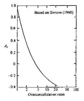
Figure 4.11 Variation of A<sub>f</sub> with overconsolidation ratio for Weald clay.
