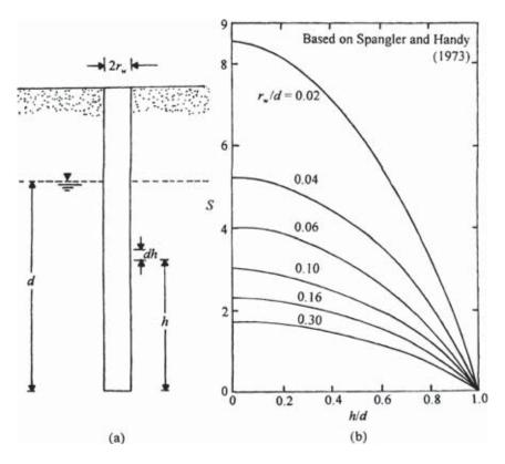
Figure 5.20 Auger hole test.
