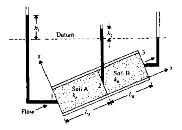
Figure 5.25 One-directional flow through two layers of soil.
