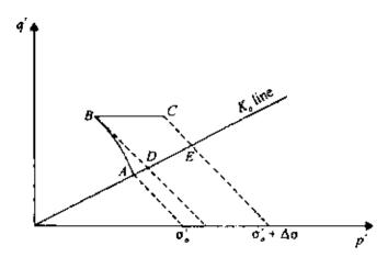
Figure 8.26 Comparison of consolidation settlement calculation procedures.
