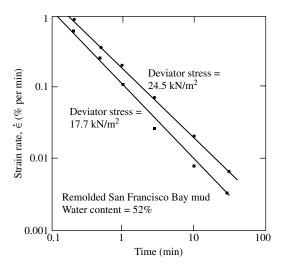
Figure 7.73 Plot of log  $\in$  versus log t during undrained creep of remolded San Francisco Bay mud (after Singh and Mitchell, 1968).
