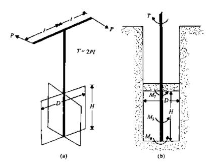
Figure 7.66 Vane shear test.
