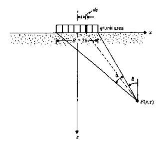
Figure 3.9 Uniform vertical loading on an infinite strip.
