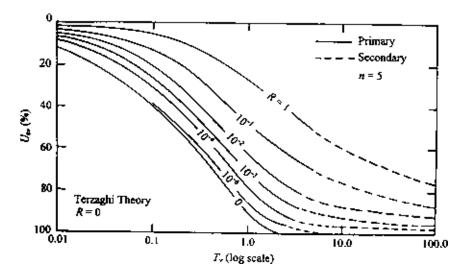
Figure 6.33 Plot of degree of consolidation versus  $T_v$  for various values of R (n = 5) (after Barden, 1965).
