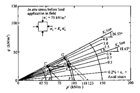
Figure 8.25 Use of stress path to calculate settlement.
