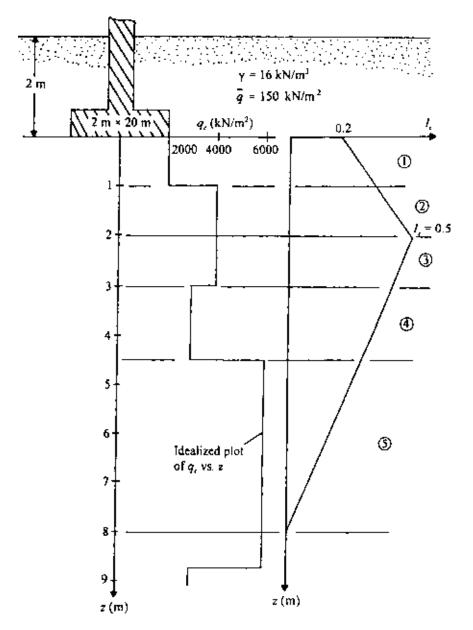
Figure 8.13 Settlement calculation under a pier foundation.
