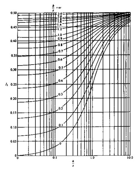
Figure 3.15 Influence factors for embankment load (after Osterberg, 1957).
