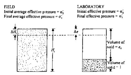
Figure 6.22 Calculation of one-dimensional consolidation settlement.
