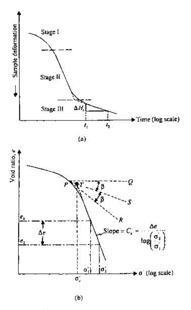
Figure 6.14 (a) Typical specimen deformation versus log-of-time plot for a given load increment and (b) Typical e versus log  $\sigma'$  plot showing procedure for determination of  $\sigma'_c$  and  $C_c$ .
