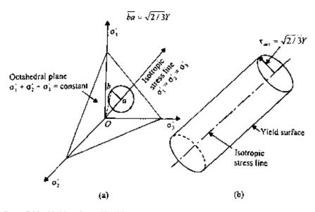
Figure 7.80 Yield surface—Von Mises criteria.
