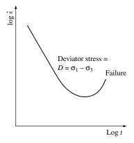
Figure 7.74 Nature of variation of log  $\dot{\in}$  versus log t for a given deviator stress showing the failure stage at large strains.
