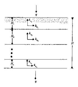
Figure 5.15 Flow in vertical direction in stratified soil.
