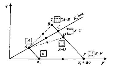
Figure 8.23 Stress path and specimen distortion.
