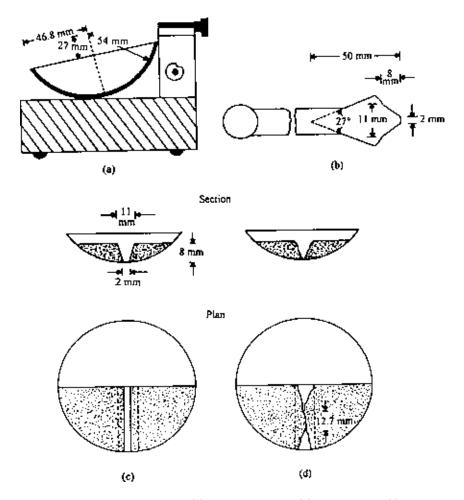
Figure 1.22 Schematic diagram of (a) liquid limit device, (b) grooving tool, (c) soil pat at the beginning of the test and (d) soil pat at the end of the test.
