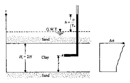
Figure 6.2 Clay layer undergoing consolidation.
