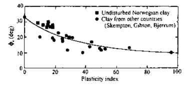
Figure 7.47 Variation of true angle of friction with plasticity index (after Bjerrum and Simons, 1960).
