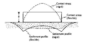
Figure 3.35 Contact pressure and settlement profiles for foundations on sand.
