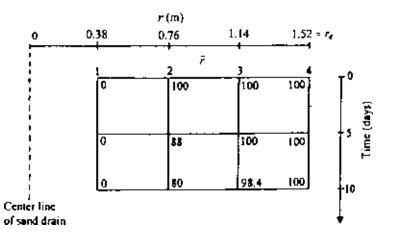
Figure 6.41 Excess pore water pressure variation with time for radial drainage.
