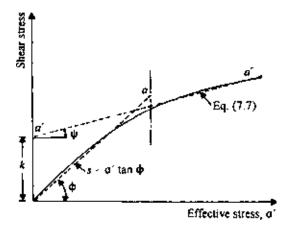
Figure 7.14 Failure envelope at high confining pressure.
