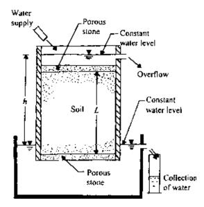
Figure 5.4 Constant-head laboratory permeability test.
