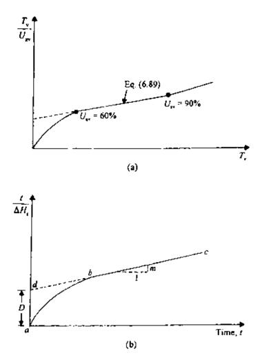
Figure 6.27 Rectangular hyperbola method for determination of  $C_v$ .
