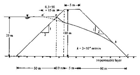
Figure 5.55 Seepage through an earth dam.
