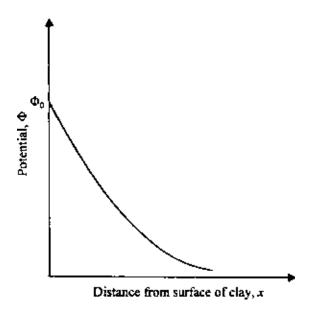
Figure 1.10 Nature of variation of potential  $\Phi$  with distance from the clay surface.
