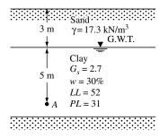
Figure 7.71 Undrained shear strength of a clay deposit.
