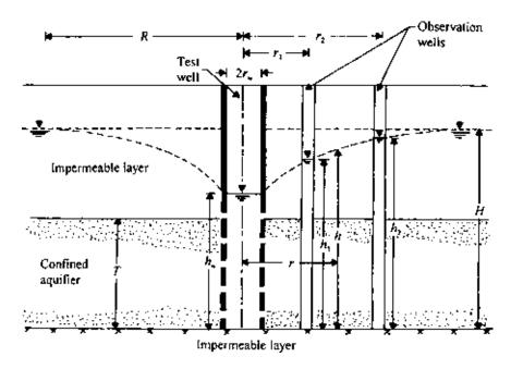
Figure 5.19 Determination of coefficient of permeability by pumping from wells confined aquifier.
