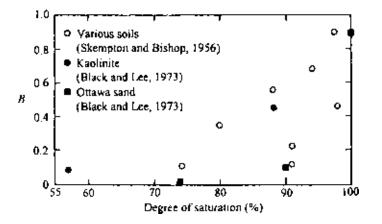
Figure 4.6 Variation of B with degree of saturation.
