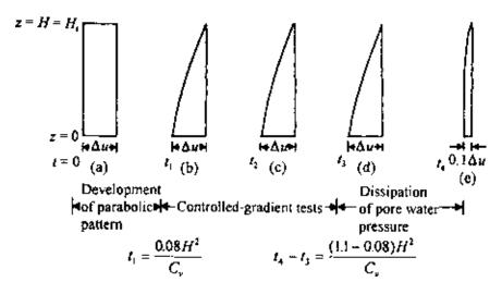
Figure 6.36 Stages in controlled-gradient test.
