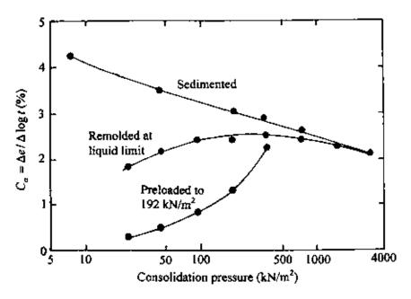
Figure 6.18 Coefficient of secondary compression for organic Paulding clay (after Mesri, 1973).
