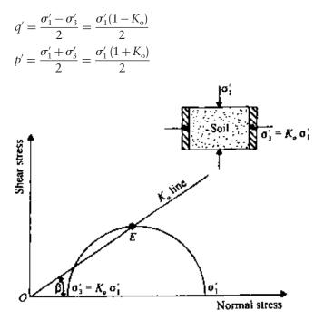
Figure 8.21 Determination of the slope of  $K_{o}$  line.
