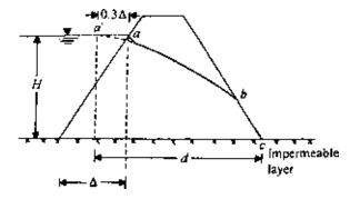
Figure 5.51 Modified distance d for use in Eq. (5.184).
