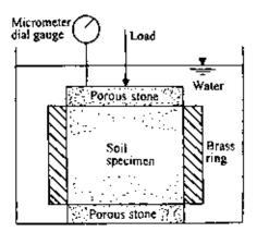
Figure 6.13 Consolidometer.
