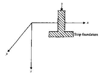
Figure 2.10 Strip foundation—plane strain problem.
