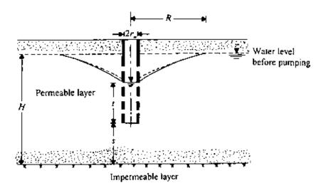
Figure 5.18 Pumping from partially penetrating gravity wells.
