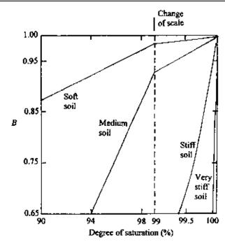
Figure 4.5 Theoretical variation of B with degree of saturation for soils described in Table 4.1 (Note: Back pressure =  $207 \text{ kN/m}^2$ ,  $\Delta \sigma = 138 \text{ kN/m}^2$ ).
