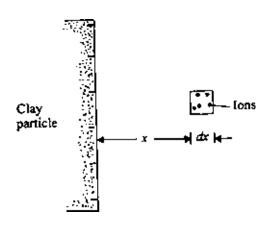
Figure 1.9 Derivation of repulsive potential equation.
