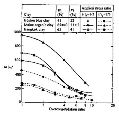
Figure 8.2 Relation between E/S<sub>u</sub> and overconsolidation ratio from consolidated undrained tests on three clays determined from CK<sub>o</sub>U type direct shear tests (after D'Appolonia et al., 1971).
