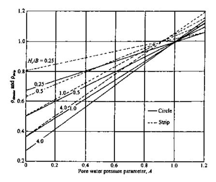
Figure 8.18 Settlement ratio for strip and circular loading.
