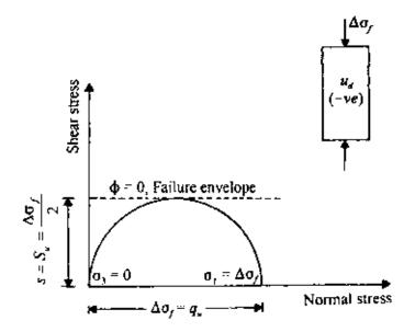
Figure 7.30 Unconfined compression strength.
