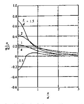
Figure 3.6 Plot of  $\sigma_z/(q/d)$  versus x/d for various values of z/d [Eq. (3.12)].
