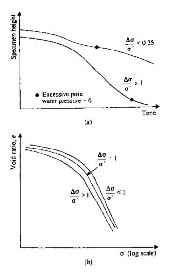
Figure 6.19 Effect of load-increment ratio.
