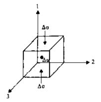
Figure 4.8 Saturated soil element under uniaxial stress increment.
