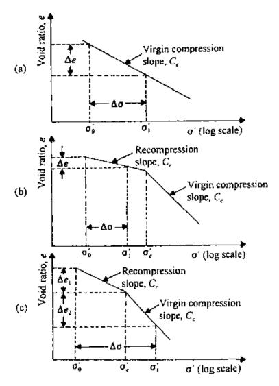
Figure 6.23 Calculation of  $\Delta e$  [Eqs. (6.77)–(6.79)].
