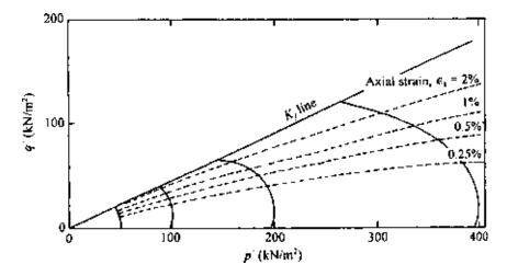
Figure 7.42 Stress path for Lagunilla clay (after Lambe, 1964).
