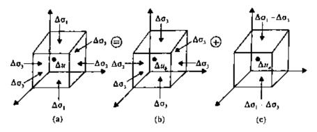
Figure 4.14 Excess pore water pressure under undrained triaxial test conditions.
