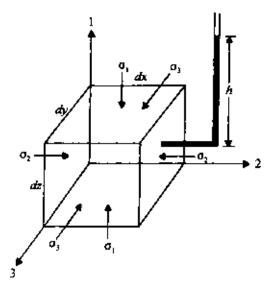
Figure 4.2 Normal total stresses in a soil mass.
