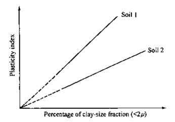
Figure 1.26 Relationship between plasticity index and percentage of clay-size fraction by weight.
