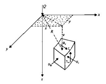
Figure 3.19 Concentrated point load (vertical) on the surface (cylindrical coordinates).
