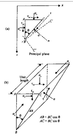
Figure 2.12 Stresses on an inclined plane for plane strain case.
