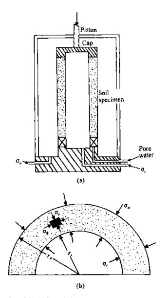
Figure 7.84 Hollow cylinder test.
