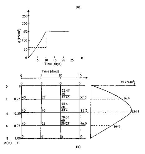
Figure 6.12 Numerical solution for ramp loading.
