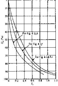
Figure 6.5 Variation of  $U_{\rm av}$  with  $T_{\rm v}$  for initial excess pore water pressure diagrams shown in Figure 6.3.
