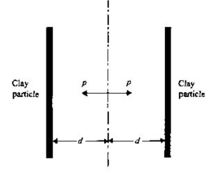
Figure 1.16 Repulsive pressure midway between two parallel clay plates.
