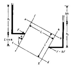
Figure 5.39 Seepage force determination.
