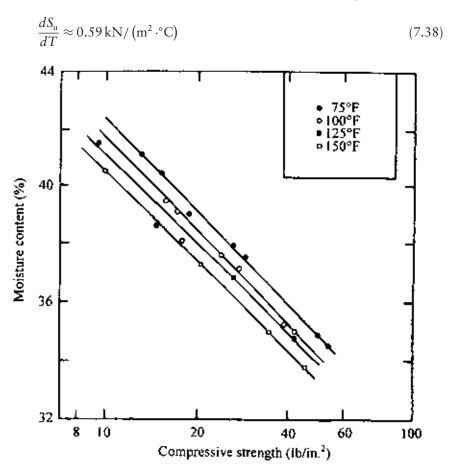
Figure 7.35 Unconfined compression strength of kaolinite—effect of temperature (After Sherif and Burrous, 1969). (Note:  $1 \text{ Ib/in.}^2 = 6.9 \text{ kN/m}^2$ .)
