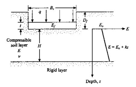
Figure 8.7 Improved equation for calculating elastic settlement—general parameters.
