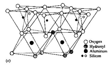
Figure 1.2 (a) Silica sheet, (b) Gibbsite sheet and (c) Silica-gibbsite sheet (after Grim, 1959).
