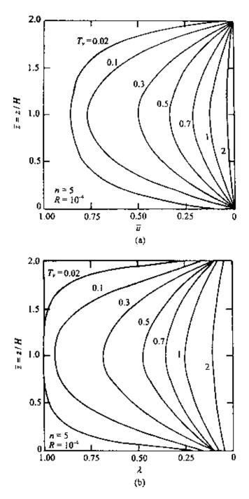
Figure 6.32 Plot of  $\bar{z}$  against  $\bar{u}$  and  $\lambda$  for a two-way drained clay layer (after Barden, 1965).
