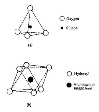
Figure 1.1 (a) Silicon–oxygen tetrahedron unit and (b) Aluminum or magnesium octahedral unit.
