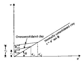
Figure 7.51 Mohr's envelope for overconsolidated clay.
