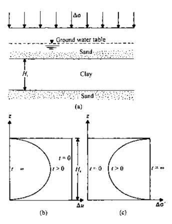
Figure 6.1 Principles of consolidation.
