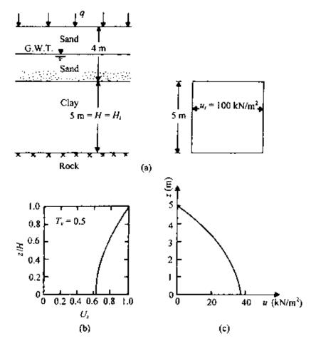
Figure 6.7 Excess pore water pressure distribution.
