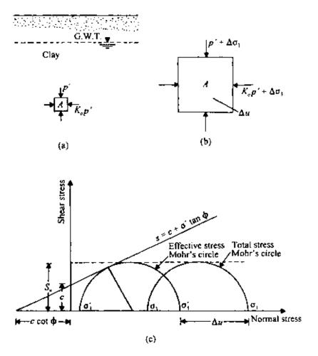
*Figure 7.69* Relation between the undrained strength of clay and the effective overburden pressure.
