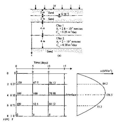
Figure 6.11 Numerical solution for consolidation in layered soil.
