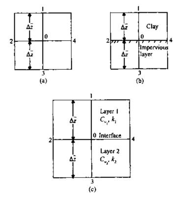
Figure 6.9 Numerical solution for consolidation.
