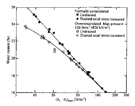
Figure 7.50 Water content versus  $(\sigma_1 - \sigma_3)_{\text{failure}}$  for Weald clay—compression tests [Note:  $I \text{ lb/in}^2 = 6.9 \text{ kN/m}^2$ ; after Henkel (1960)].
