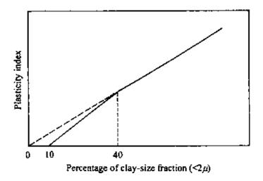
Figure 1.28 Simplified relationship between plasticity index and percentage of claysize fraction by weight (after Seed *et al.*, 1964b).
