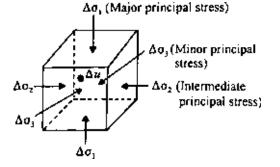
Figure 4.15 Saturated soil element with major, intermediate, and minor principal stresses.
