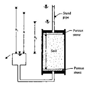
Figure 5.5 Falling-head laboratory permeability test.
