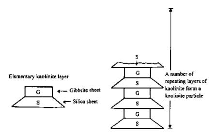
Figure 1.3 Symbolic structure for kaolinite.
