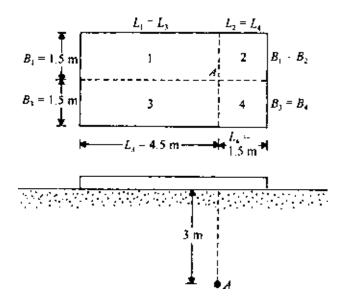
Figure 3.27 Distributed load on a flexible rectangular area.
