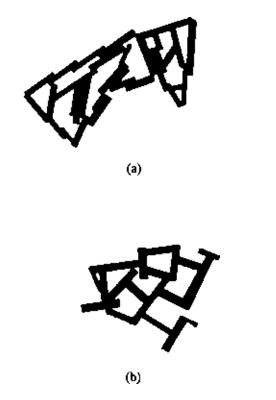
Figure 1.20 (a) Salt and (b) nonsalt flocculation of clay particles.
