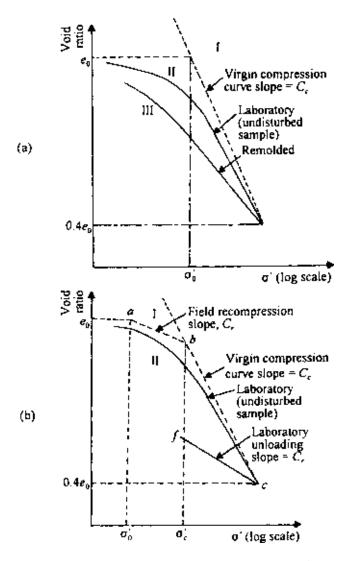
Figure 6.16 Effect of sample disturbance on e versus  $\log \sigma'$  curve.
