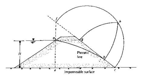
Figure 5.50 Graphical construction for Schaffernak's solution.
