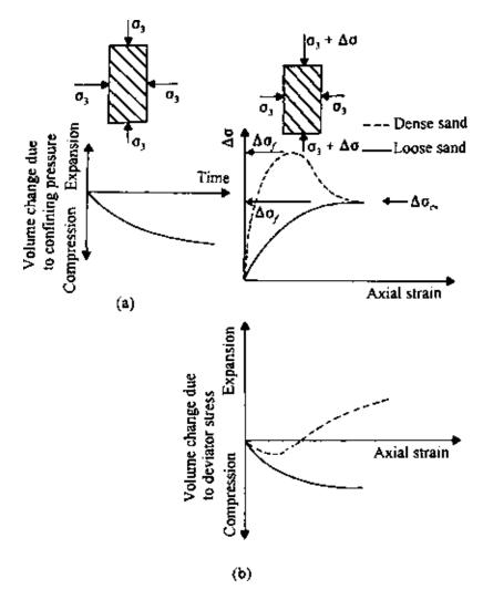
Figure 7.8 Drained triaxial test in granular soil (a) Application of confining pressure and (b) Application of deviator stress.
