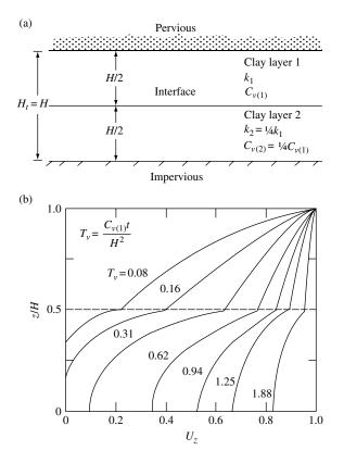
Figure 6.10 Degree of consolidation in two-layered soil [Part (b) after Luscher, 1965].
