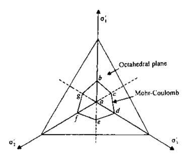
Figure 7.82 Mohr-Coulomb failure criteria.
