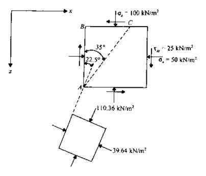
Figure 2.17 Determination of principal stresses at a point.
