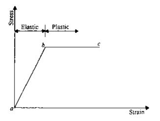
Figure 2.1 Idealized stress-strain diagram.
