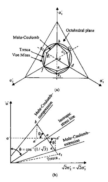
Figure 7.83 Comparison of Von Mises, Tresca, and Mohr–Coulomb yield functions.
