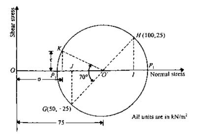
Figure 2.18 Mohr's circle for stress determination.
