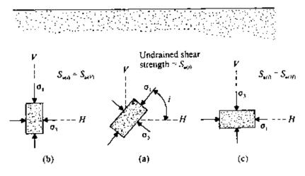
*Figure 7.56* Strength anisotropy in clay.
