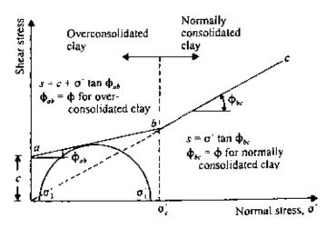
Figure 7.22 Failure envelope of a clay with preconsolidation pressure of  $\sigma'_{\rm c}$ .
