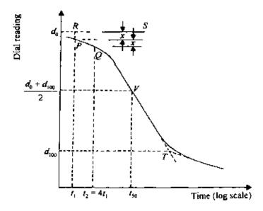
*Figure 6.24* Logarithm-of-time method for determination of  $C_{y}$ .
