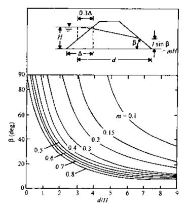
*Figure 5.53* Chart for solution by L. Casagrande's method based on Gilboy's solution.
