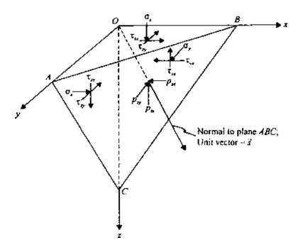
Figure 2.20 Stresses on an inclined plane—three-dimensional case.
