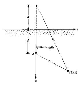
Figure 3.5 Vertical line load inside a semi-infinite mass.
