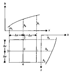
Figure 5.36 Hydraulic heads for flow in a region.
