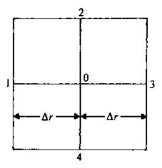
Figure 6.40 Numerical solution for radial drainage.
