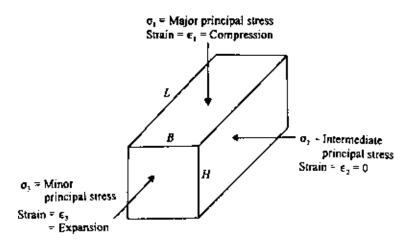
Figure 7.15 Plane strain condition.
