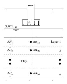
Figure 8.15 Calculation of consolidation settlement-method B.
