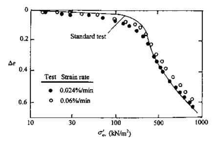
Figure 6.34 CRS tests on Messena clay—plot of  $\Delta e$  versus  $\sigma'_{av}$  (after Smith and Wahls, 1969).
