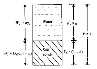
Figure 1.34 Weight-volume relationship for saturated soil with V = I.
