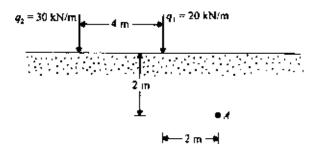
Figure 3.3 Two line loads acting on the surface.
