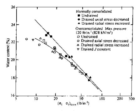
*Figure 7.49* Water content versus  $(\sigma_1 - \sigma_3)_{\text{failure}}$  for Weald clay—extension tests [*Note:* 1 lb/in<sup>2</sup> = 6.9 kN/m<sup>2</sup>; after Henkel (1960)].
