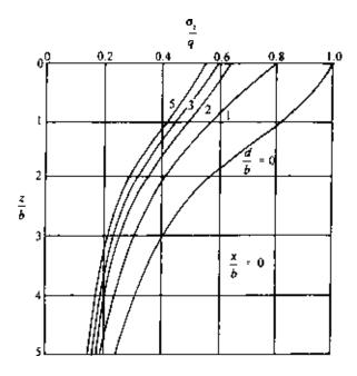
Figure 3.11 Plot of  $\sigma_z/q$  versus z/b [Eq. (3.33)].
