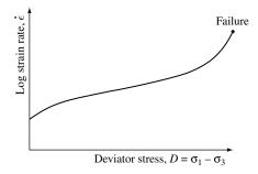
Figure 7.75 Variation of the strain rate  $\dot{\in}$  with deviator stress at a given time t after the start of the test.
