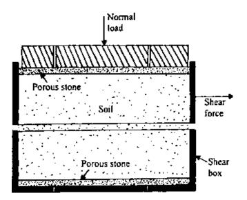
Figure 7.2 Direct shear test arrangement.
