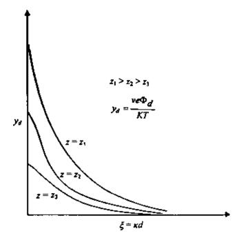
Figure 1.15 Nature of variation of the nondimensional midplane potential for two parallel plates.
