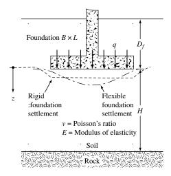
Figure 8.3 Elastic settlement of flexible and rigid foundations.
