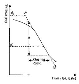
Figure 6.26 Maximum-slope method for determination of  $C_{v}$ .
