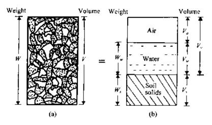
Figure 1.30 Weight-volume relationships for soil aggregate.
