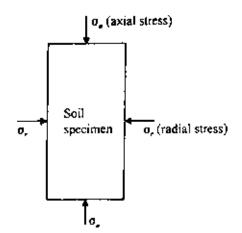
Figure 7.10 Soil specimen subjected to axial and radial stresses.
