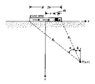
Figure 3.12 Uniform horizontal loading on an infinite strip.
