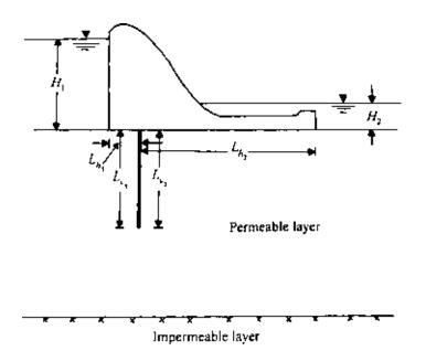
Figure 5.41 Calculation of weighted creep distance.
