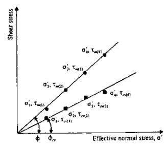
Figure 7.4 Determination of peak and ultimate friction angles from direct shear tests.
