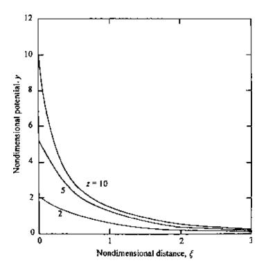
Figure 1.11 Variation of nondimensional potential with nondimensional distance.
