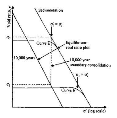
Figure 6.21 Effect of secondary consolidation.
