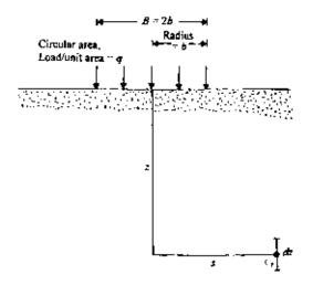
Figure 3.23 Elastic settlement due to a uniformly loaded circular area.
