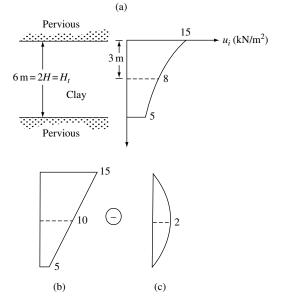
*Figure 6.6* Calculation of average degree of consolidation ( $T_v = 0.3$ ).
