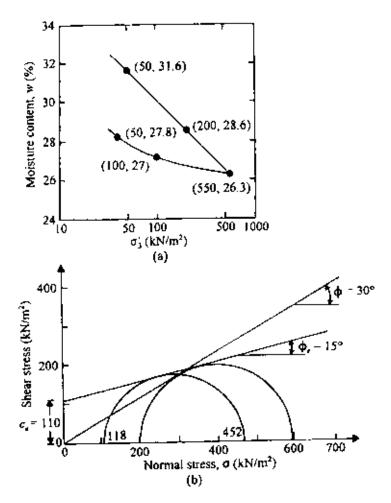
Figure 7.48 Determination of Hvorslev's parameters.
