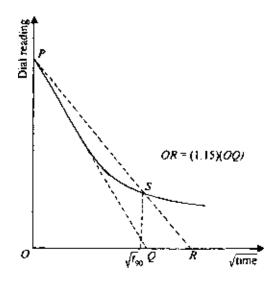
*Figure 6.25* Square-root-of-time method for determination of  $C_{y}$ .
