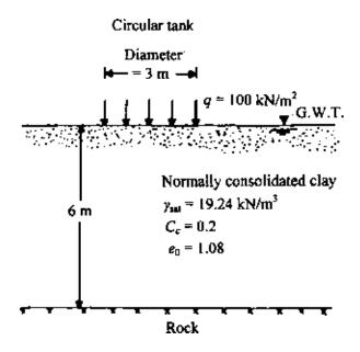
Figure 8.19 Consolidation settlement under a circular tank.
