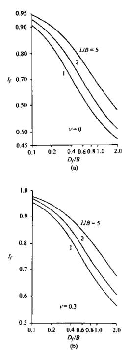
Figure 8.4 Variation of  $I_f$  with  $D_f/B$ , L/B, and  $\nu$ .
