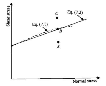
Figure 7.1 Mohr–Coulomb failure criteria.
