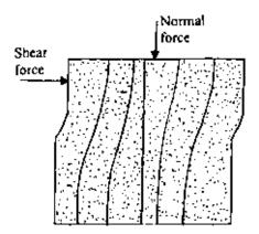
Figure 7.5 Unequal stress distribution in direct shear equipment.
