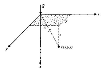
Figure 3.18 Concentrated point load on the surface (rectangular coordinates).
