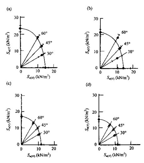
Figure 7.59 Vane shear strength polar diagrams for a soft marine clay in Thailand. (a) Depth = 1 m; (b) depth = 2 m; (c) depth = 3 m; (d) depth = 4 m (after Richardson et al., 1975).
