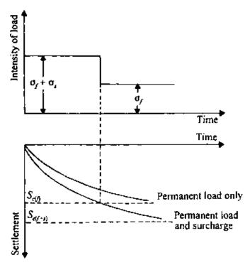
Figure 8.27 Concept of precompression technique.
