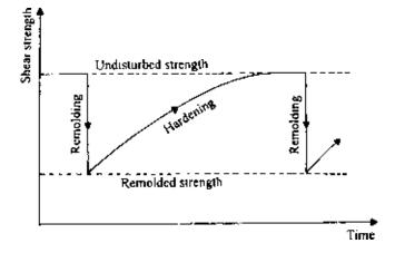
Figure 7.60 Thixotropy of a material.
