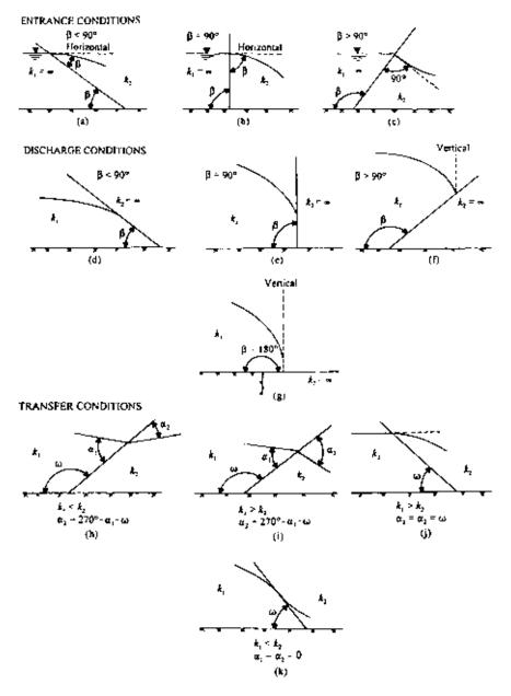
Figure 5.59 Entrance, discharge, and transfer conditions (after Casagrande, 1937).
