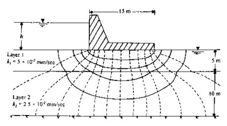
Figure 5.35 Flow net under a dam resting on a two-layered soil deposit.
