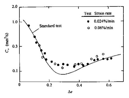
Figure 6.35 CRS tests on Messena clay—plot of  $C_v$  versus  $\Delta e$  (after Smith and Wahls, 1969).
