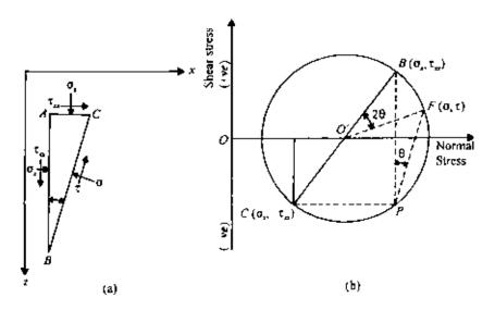
Figure 2.16 Pole method of finding stresses on an inclined plane.
