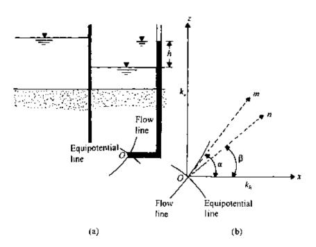
Figure 5.11 Directional variation of coefficient of permeability.
