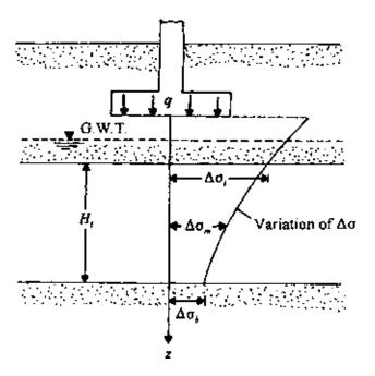
Figure 8.14 Calculation of consolidation settlement—method A.
