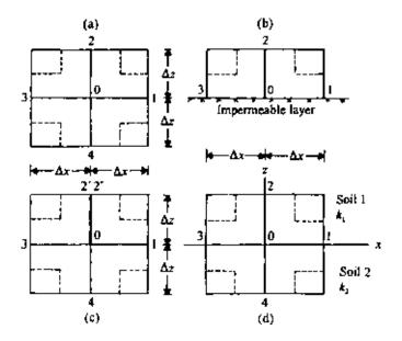
Figure 5.37 Numerical analysis of seepage.
