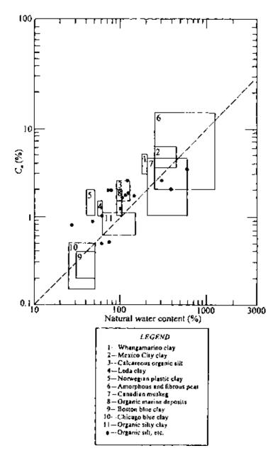
Figure 6.17 Coefficient of secondary consolidation for natural soil deposits (after Mesri, 1973).
