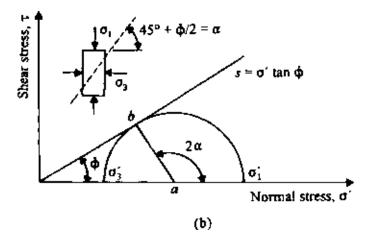
Figure 7.9 Drained triaxial test results.
