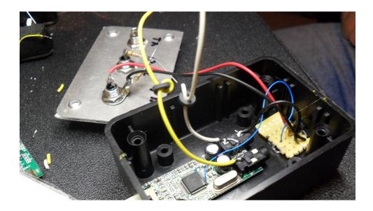
Note that half way up the yellow and white wire we have placed a ferrite bead for RF suppression.
