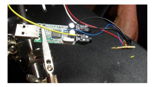
On the bottom connector we solder a wire (yellow in our photo) to the upper left corner of the phone jack.
