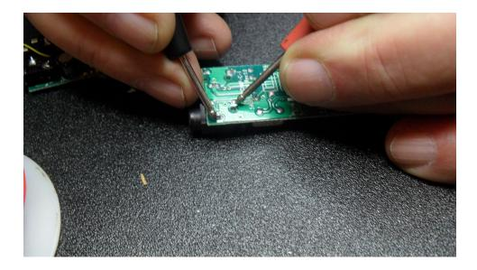
Now is the biggest challenge of the project. We must solder a piece of tiny (wire wrap) wire, to pin 13 on the IC located in the center of the FOB. You will note that pin 13 is on the corner of the chip, which is good for soldering. I would suggest you use the largest magnifying glass you have along with the smallest solder station and tip. Also, have some solder wick available in the event you bridge some of the pins with solder. If that should happen, use the wick to clean the pins.
