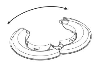
Wrap escutheon ring (A) around extension column and snap into place to cover hole in ceiling tile.
