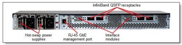
Figure 4. Rear view of the FlashSystem unit with the InfiniBand interfaces
