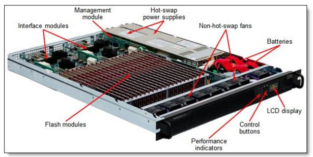
Figure 2 shows the internal components of the FlashSystem unit.
